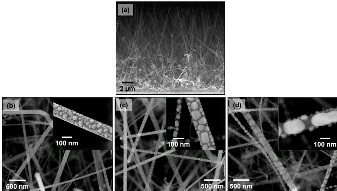
**Figure S1.** (a) Low magnification cross-sectional SEM micrograph of the as-grown uncoated SiNWs. Plan-view SEM images of the as-synthesized nanowires with high magnification inserts. (b) 1Sn/SiNWs, (c) 3Sn/SiNWs, and (d) 5Sn/SiNWs.
