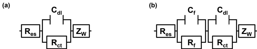
**Figure S3.** Equivalent circuits used for fitting impedance spectra of (a) as-synthesized bare and coated SiNWs, and (b) post-100 cycles (at 0.1C) bare and coated SiNWs.
