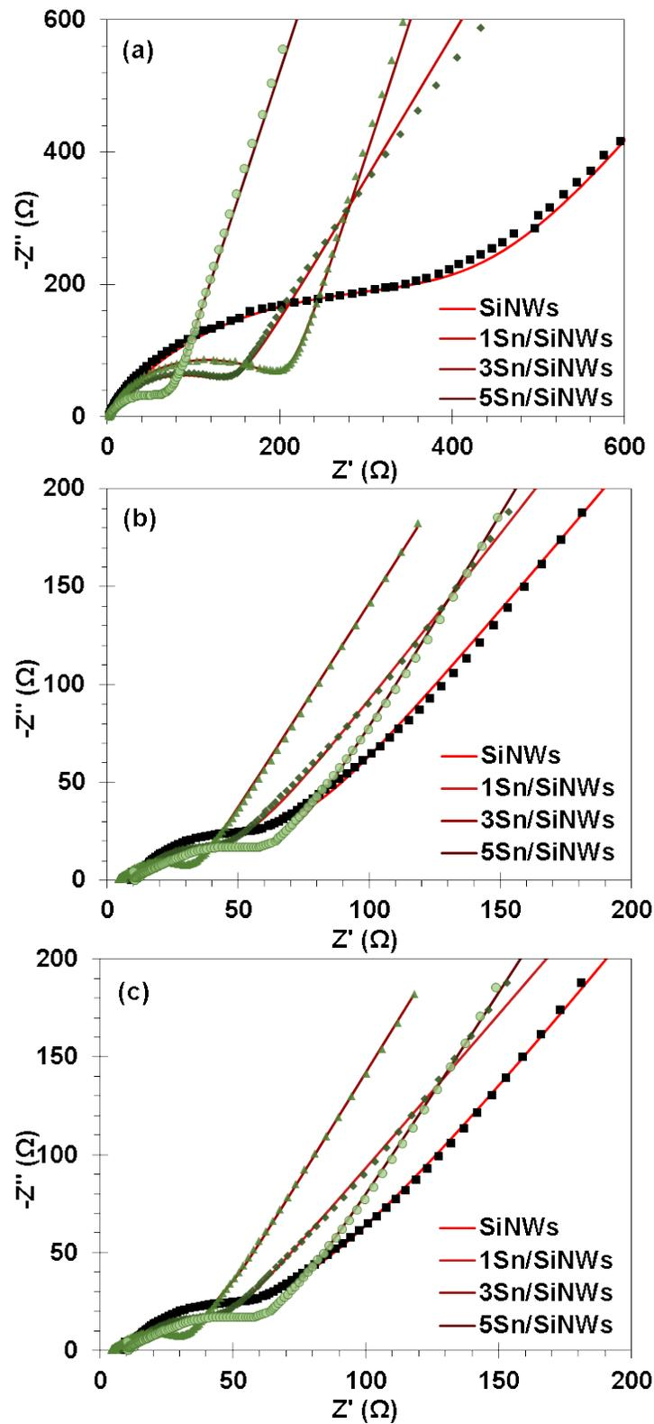
**Figure S4.** The measured and modeled EIS plots for (a) as-synthesized and (b,c) post 100 cycles at 0.1C anode materials. Modeled data obtained from using the equivalent circuit shown in (a,b) Figure S3(a) and (c) Figure S3(b).
