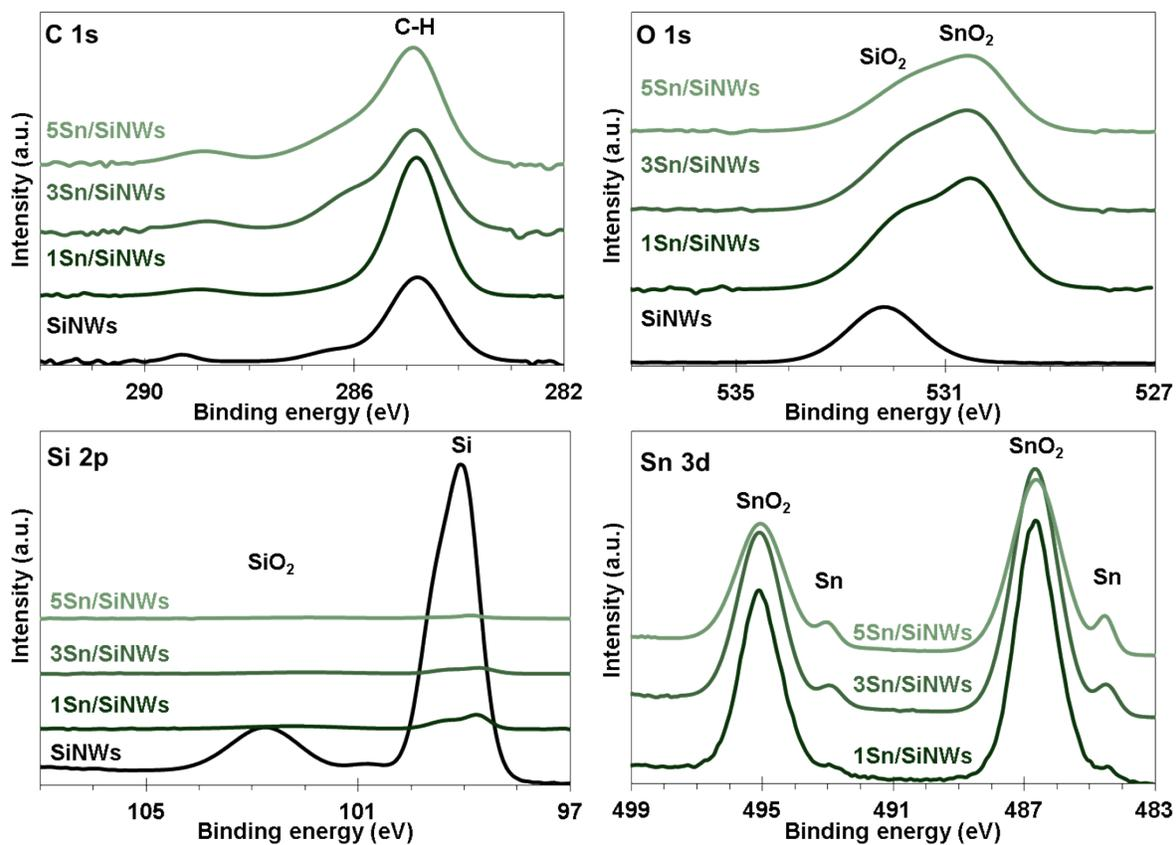
**Figure S2.** C 1s, O 1s, Si 2p, and Sn 3d XPS spectra for as-prepared SiNWs, 1Sn/SiNWs, 3Sn/SiNWs, and 5Sn/SiNWs.
