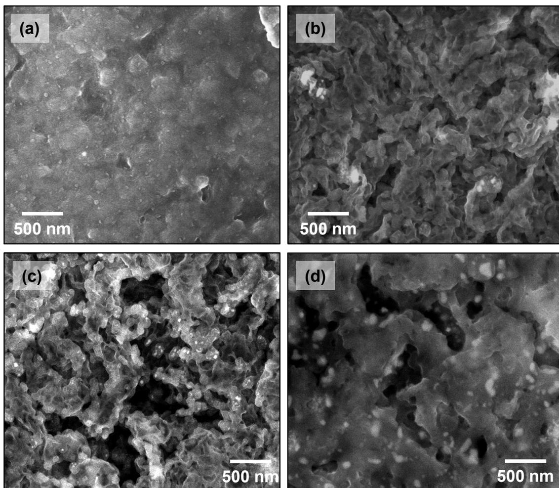
**Figure S5.** Plan-view SEM micrographs of (a) SiNWs, (b) 1Sn/SiNWs, (c) 3Sn/SiNWs, and (d) 5Sn/SiNWs anode materials after 100 cycles at 0.1C.
