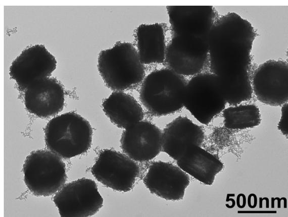
**Figure S5** TEM image of hollow Cr(OH)<sub>3</sub> hexagonal pellet prepared by the reaction of 50 ml 10 mM CrCl<sub>3</sub> solution and 0.064g NaBH<sub>4</sub>(solid) for 12 hours
