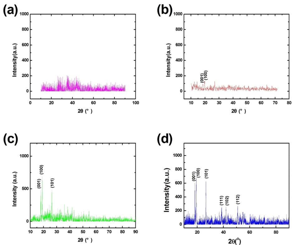
**Figure S2** XRD patterns of the products after different time of reaction. (a)1 second, (b)15 seconds, (c)1 day ,(d)5 days
