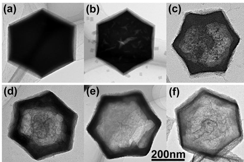
**Figure S3** TEM images of  $\text{Cr}(\text{OH})_3$  hexagonal pellets after different reaction times. (a)0.5day, (b)1 day, (c)2days, (d)3 days, (e)4 days, (f)5days.
