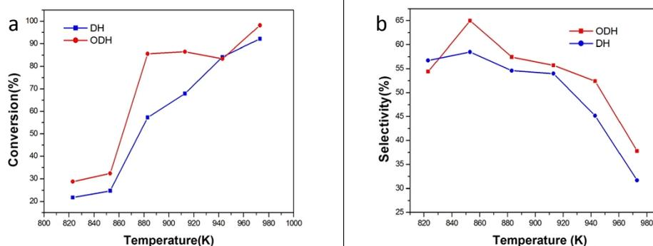
**Figure S7** Isobutane conversion (a) and the Isobutene selectivity (b) of  $i\text{-C}_4\text{H}_{10}$  as a function of temperature in oxidative dehydrogenation (ODH) and direct dehydrogenation (DH) reactions.
