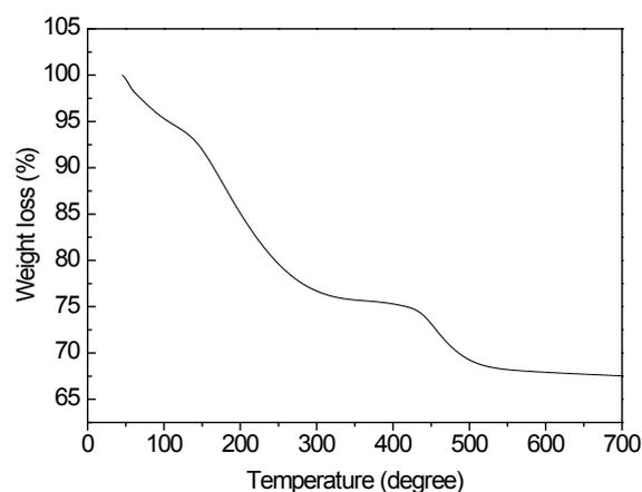
**Figure S1** the TGA (thermal gravimetric analysis) curve of as-prepared product from Room Temperature to 700 °C
