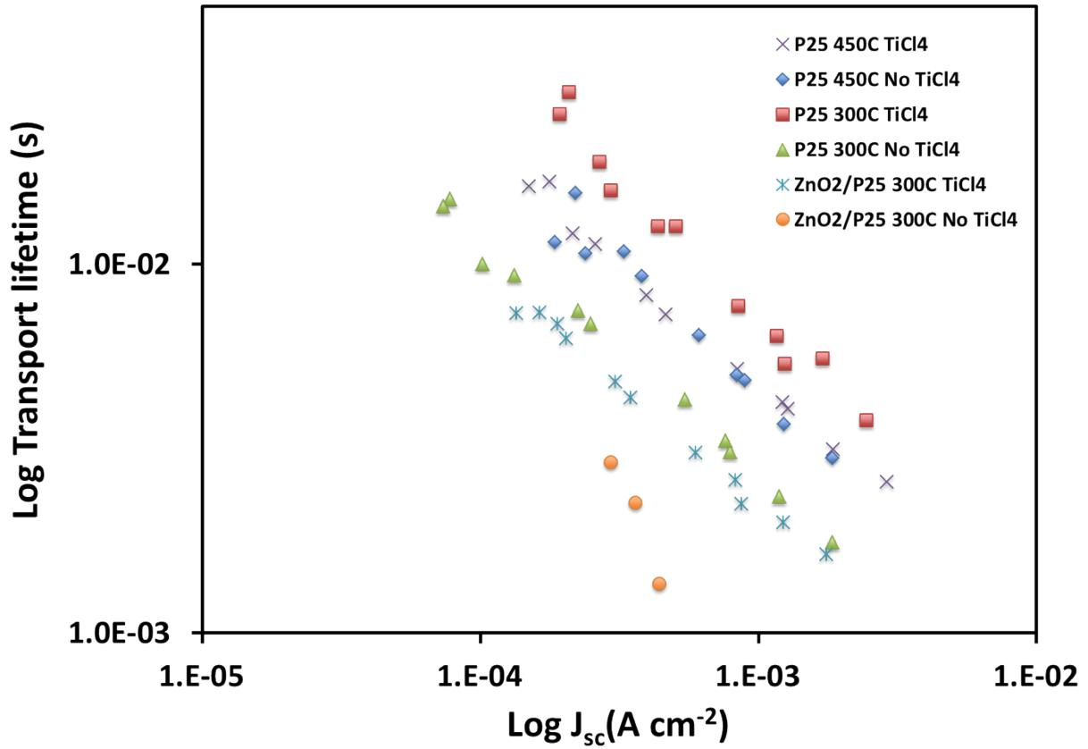
**ESI Fig. 5** Log transport time *versus* Log  $J_{sc}$  for various devices as shown. Data calculated from transient photo-current measurements
