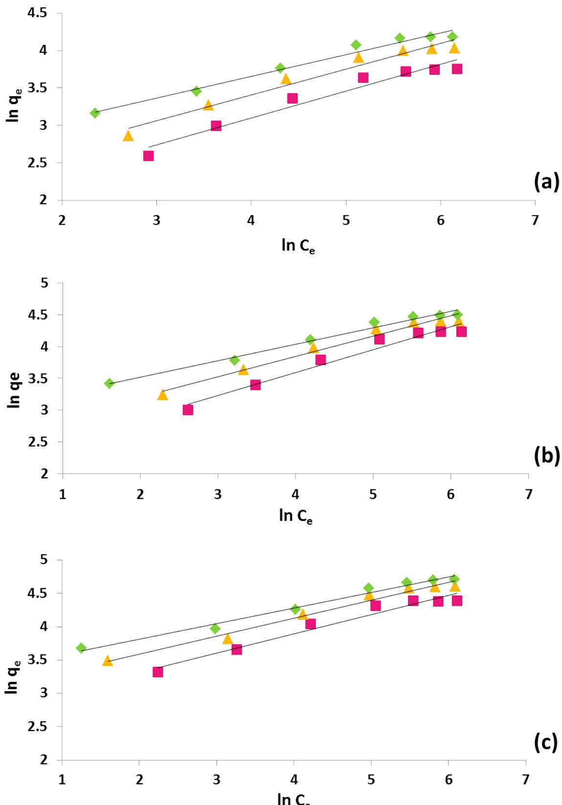
**ESI Fig. 11** Adsorption data fitted to Freundlich isotherms for N719 dye uptake on P25 films sintered at 450 °C (red squares) and onto P25/ZnO<sub>2</sub> films sintered either at 450 (green diamonds) or 300 °C (yellow triangles). Dyeing temperatures were (a) 22, (b) 40 or (c) 50 °C.
