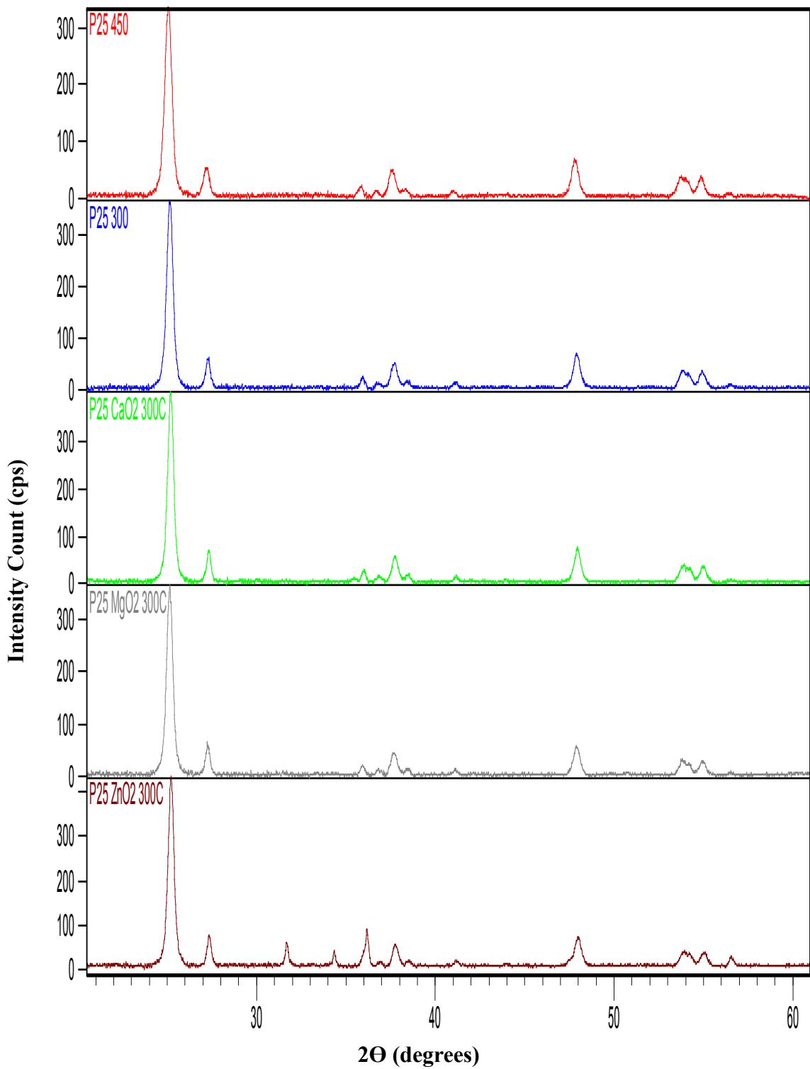
**ESI Fig. 6** XRD data for a P25 film sintered at 450 °C or at 300 °C for 30 min and for P25/CaO<sub>2</sub>, P25/MgO<sub>2</sub> and P25/ZnO<sub>2</sub> films after sintering at 300 °C for 30 min.
