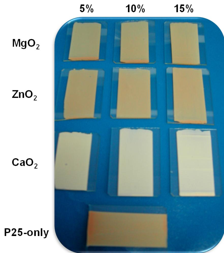
**ESI Fig. 3** Photograph of films (*ca.* 4x2 cm) prepared from P25 and P25/peroxides (5-15% w/w) binder-containing pastes after sintering for 30 min at 250 °C
