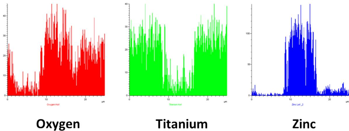
**ESI Fig. 8** SEM image of particle on surface of P25 film. Yellow line ( $25 \mu\text{m}$ ) denotes line of EDX analysis with data for oxygen (red), titanium (green) and zinc (blue) shown underneath.
