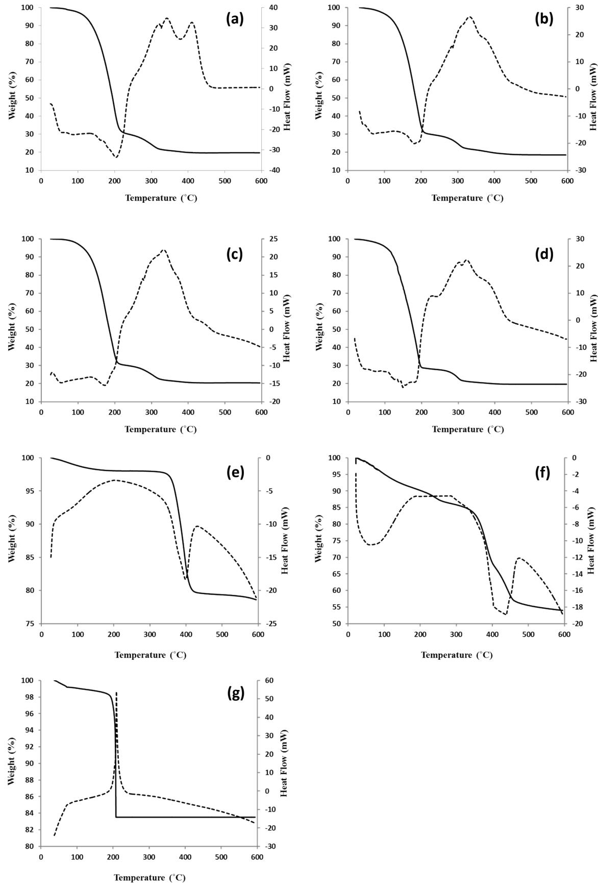
**ESI Fig. 2** TGA (solid line) and DSC (dashed line) of (a) P25, (b) P25/CaO<sub>2</sub>, (c) P25/MgO<sub>2</sub> and (d) P25/ZnO<sub>2</sub> pastes along with (e) CaO<sub>2</sub>, (f) MgO<sub>2</sub> and (g) ZnO<sub>2</sub> powders
