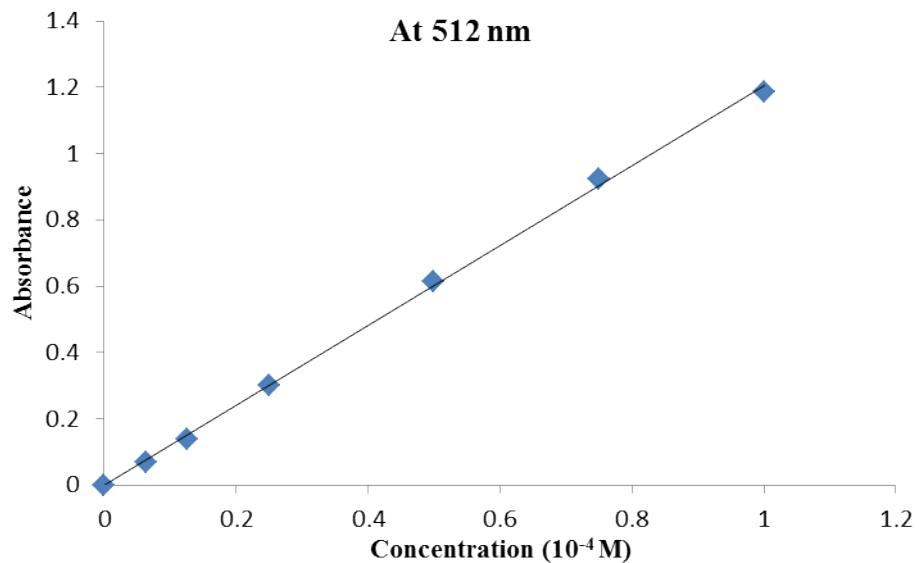
**ESI Fig. 1** Calibration curves of N719 dye in mixture solution of 0.1M NaOH<sub>(aq)</sub>/ ethanol at 1:1 (v/v) at different concentrations ( $0.0625 \times 10^{-4}$ - $1 \times 10^{-4}$ ) M in 376 and 512 nm.
