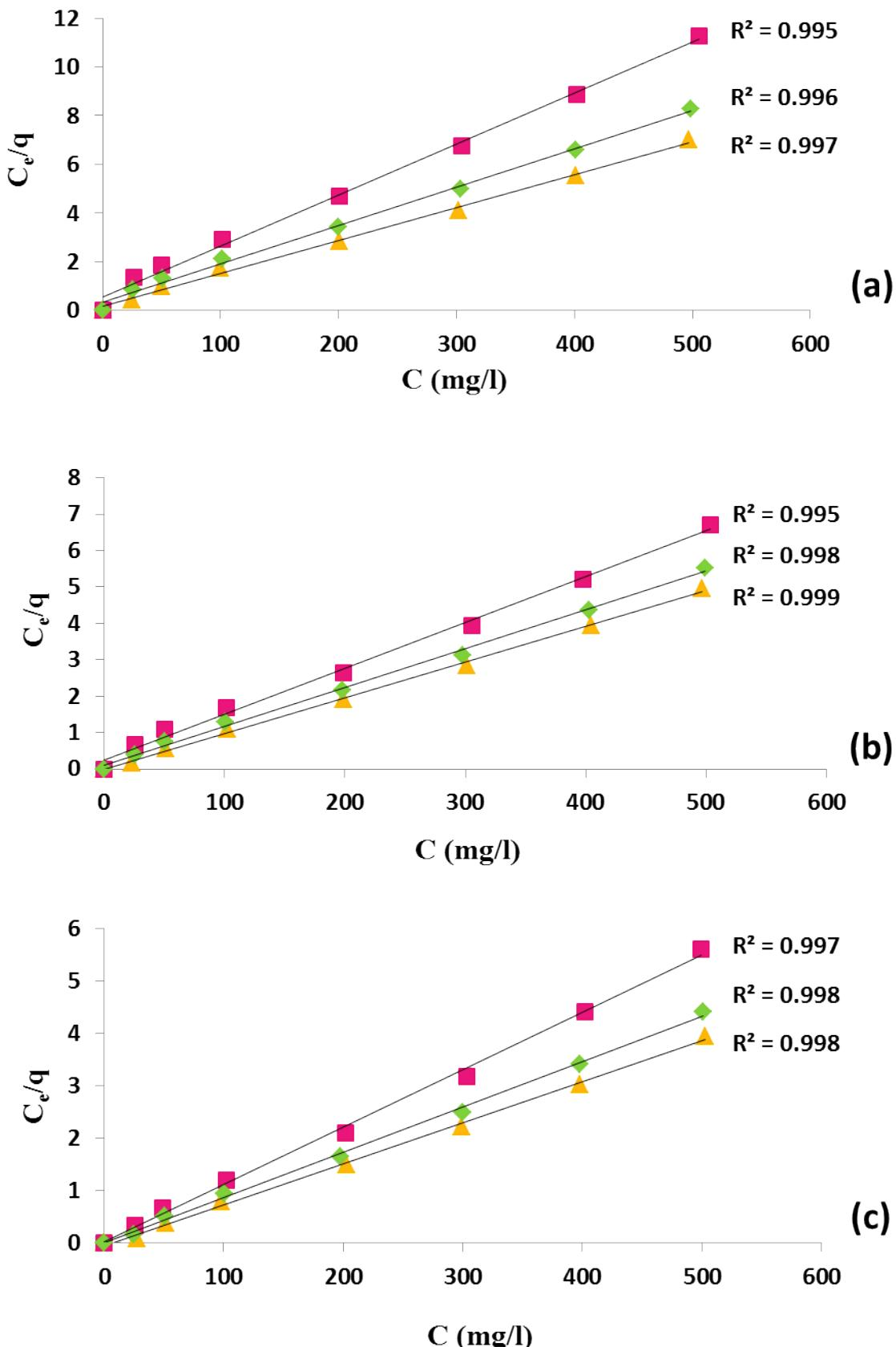
**ESI Fig. 10** Adsorption data fitted to Langmuir isotherms for N719 dye uptake on P25 films sintered at 450 °C (red squares) and onto P25/ZnO<sub>2</sub> films sintered either at 450 (green diamonds) or 300 °C (yellow triangles). Dyeing temperatures were (a) 22, (b) 40 or (c) 50 °C.
