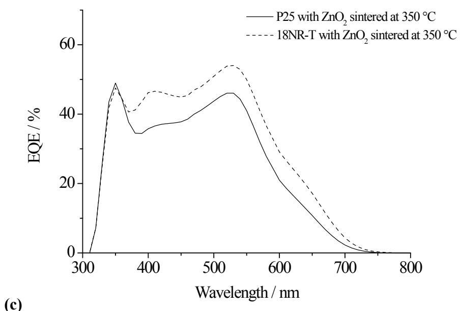
**ESI Fig. 4** (a) Photographs of N719-dyed devices for P25 paste (left) and higher dye loading on DSL18NR-T device (right) and EQE of devices sintered at (b) 450 °C or (c) 350 °C
