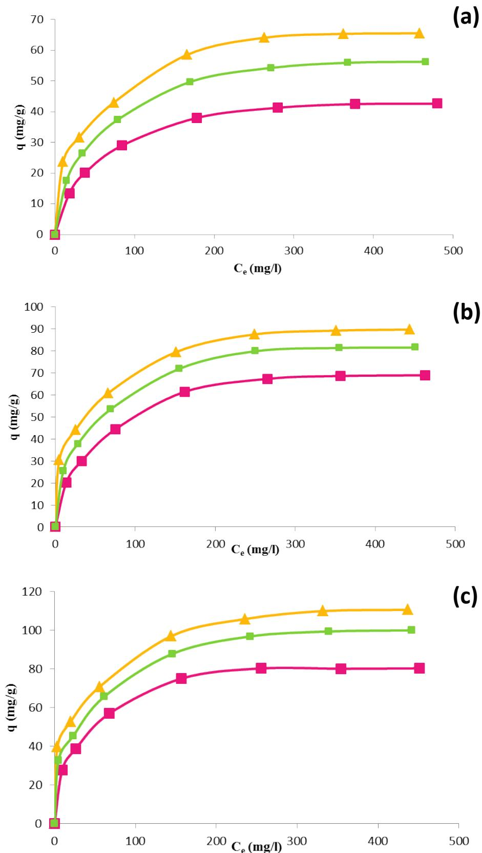
**ESI Fig. 9** Adsorption isotherms for N719 on P25 films sintered at 450°C (red lines), and also onto P25/ZnO<sub>2</sub> films sintered at either 450 (green lines) or 300°C (yellow lines). Dyeing temperature was (a) 22, (b) 40 or (c) 50°C.
