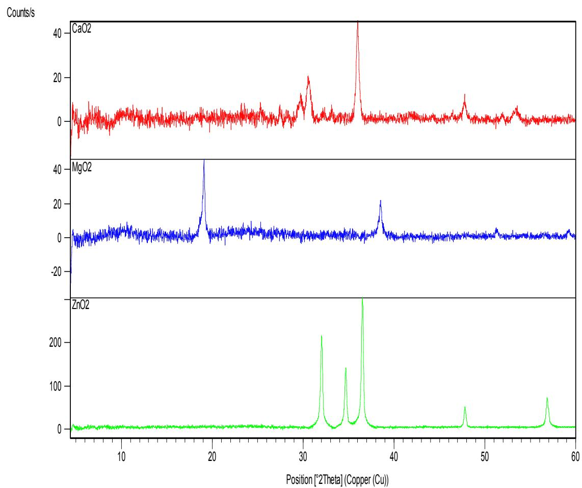
**ESI Fig. 7** XRD data for a  $\text{CaO}_2$ ,  $\text{MgO}_2$  and  $\text{ZnO}_2$  powders sintered at  $300^{\circ}\text{C}$  for 30 min.
