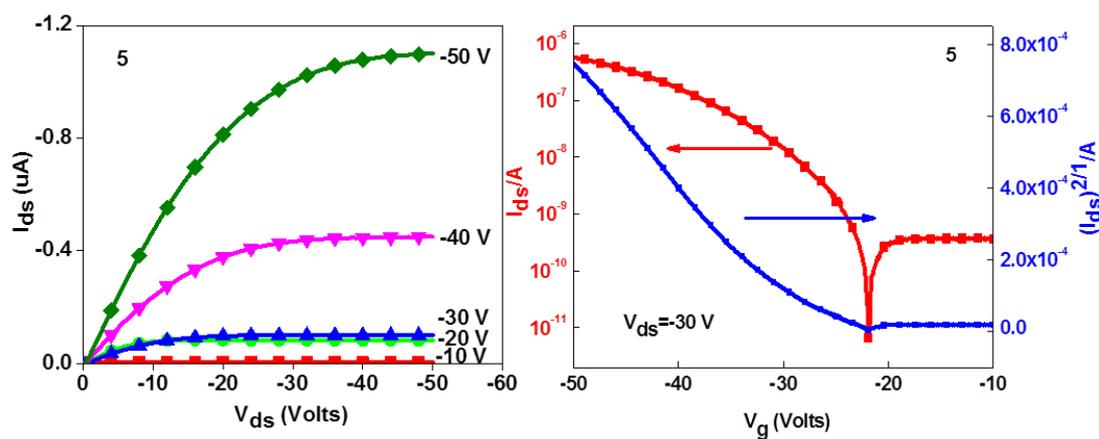
**Figure S40.** The Output (left) and Transfer (right) curves of **5** FETs with PMMA modified Si/SiO<sub>2</sub> substrate.
