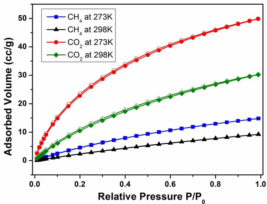
**Fig. S4.** CO<sub>2</sub> and CH<sub>4</sub> adsorption (solid circles) and desorption (open circles) isotherms of PAF-41.
