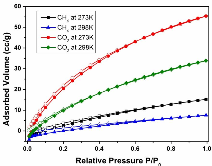
**Fig. S5.** CO<sub>2</sub> and CH<sub>4</sub> adsorption (solid circles) and desorption (open circles) isotherms of PAF-42.
