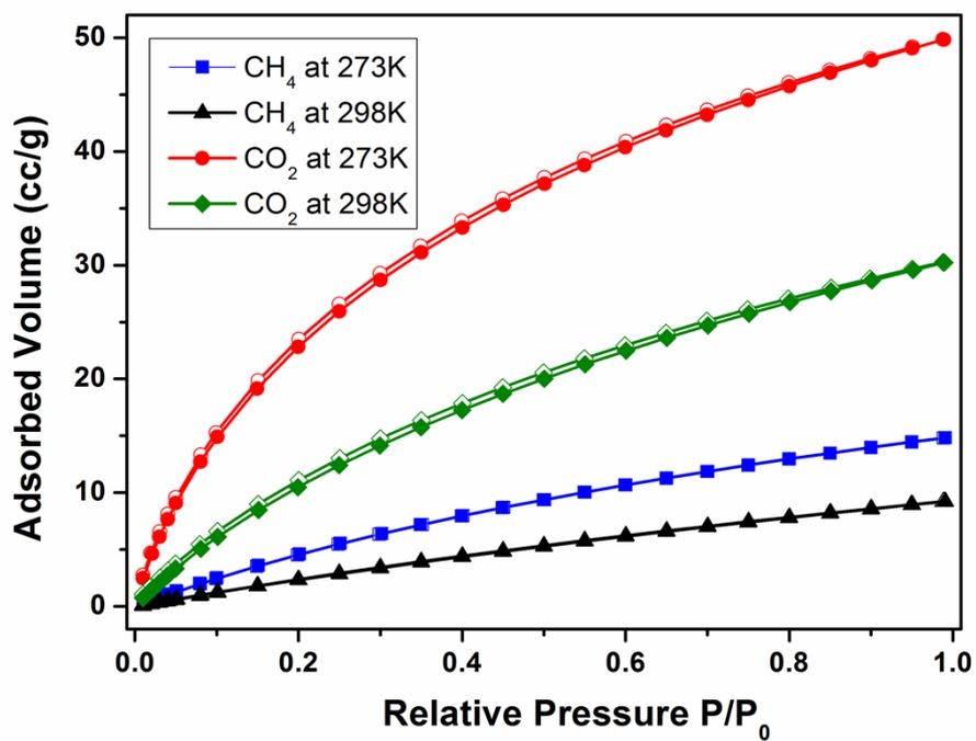
**Fig. S7.** CO<sub>2</sub> and CH<sub>4</sub> adsorption (solid circles) and desorption (open circles) isotherms of PAF-44.
