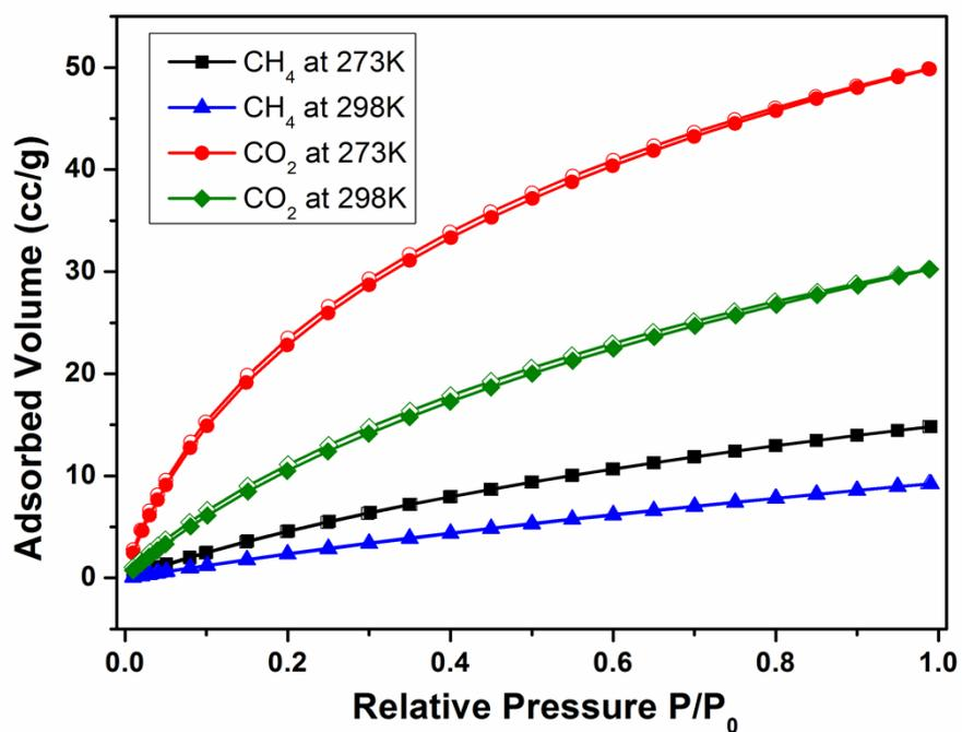
**Fig. S6.** CO<sub>2</sub> and CH<sub>4</sub> adsorption (solid circles) and desorption (open circles) isotherms of PAF-43.
