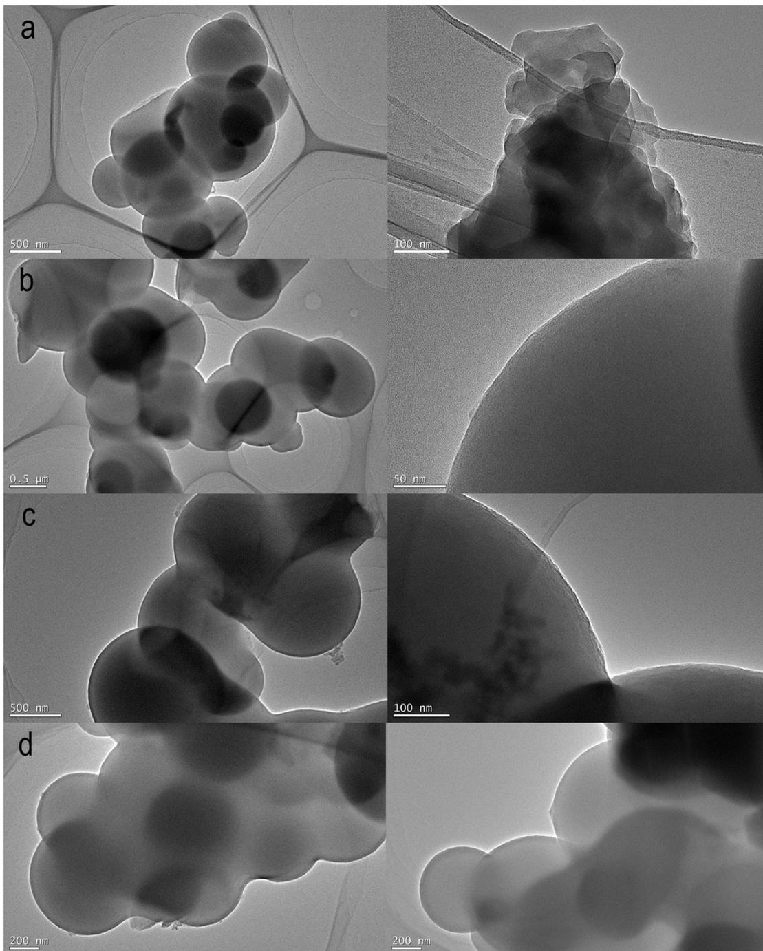
**Fig. S3.** TEM images of PAF-41 (a), PAF-42 (b), PAF-43 (c) and PAF-44 (d).
