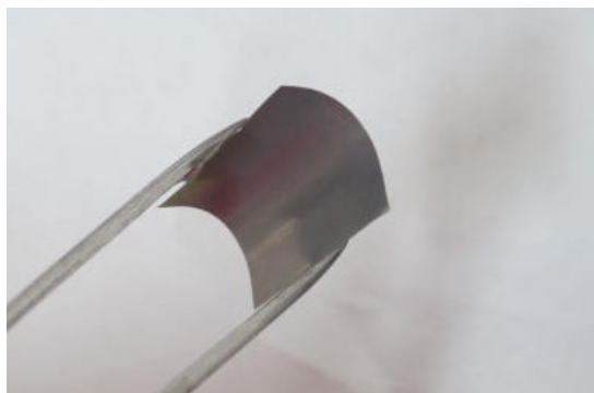
Fig. S1 Digital photo of ZnCo-LDH-100 film directly grown on a flexible Ni foil
