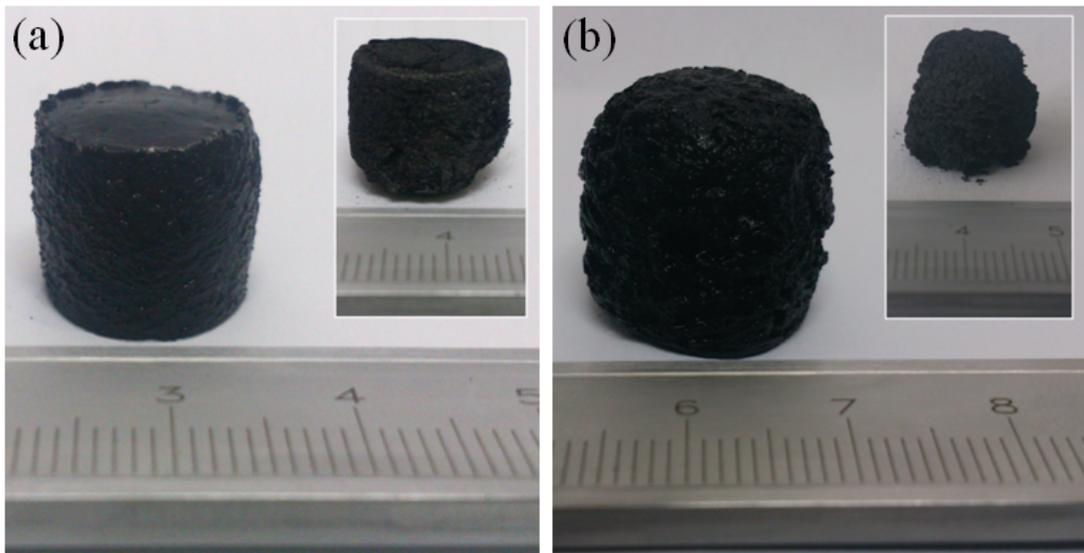
Fig. S1. (a) Photographs of UTO/GH before freeze drying and UTO/GF after freeze drying (Inset);
