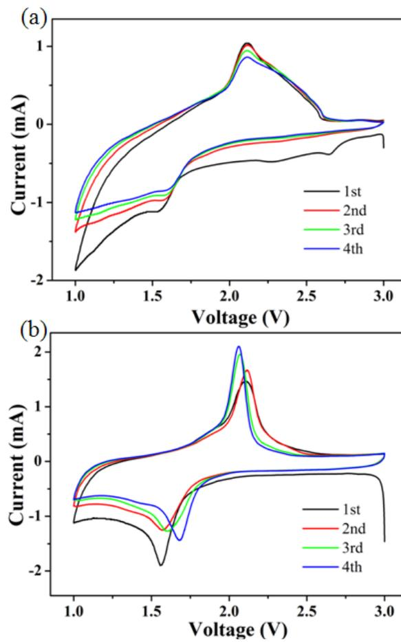
Fig. S4. Cyclic voltammograms of (a) UTO and (b) UTO/GF electrode between 1.0 and 3.0 V at a scan rate of  $0.5 \text{ mV s}^{-1}$  for the first four cycles.
