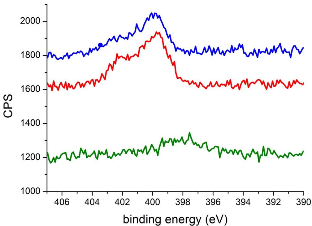
**Figure 3:** XPS narrow scan spectrum of the N1s signal of the bare particles ((1), green), the APTES particles ((2), red curve) and the CD covered particles ((4), blue curve).
