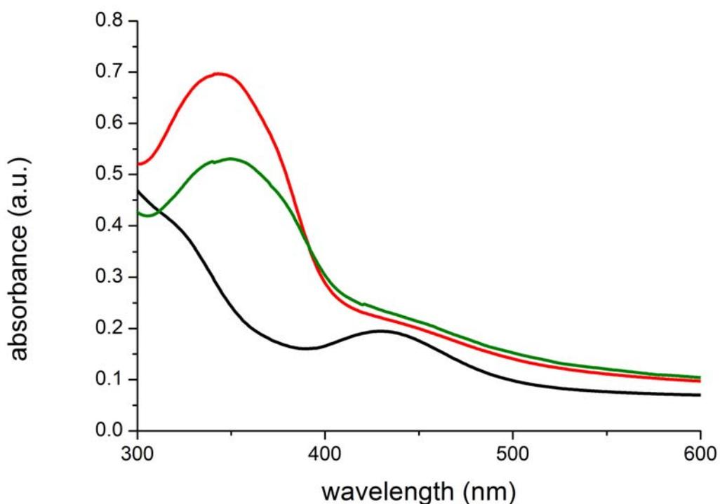
**Figure S11:** UV-vis spectra of  $\beta$ -CD-NH-NP (**4**) ( $c = 0.085$  mg/mL) in phosphate buffer after addition of the azobenzene linker (**6**) ( $c = 20\mu\text{M}$ ): Before (*trans*, red curve), after UV light irradiation ( $\lambda = 365$  nm) for 20 min (*cis*, black curve) and after visible light irradiation ( $\lambda = 455$  nm) for 20 min (*retrans*, green curve).
