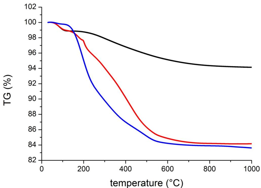
**Figure S7:** TGA curves of the bare particles ((1), black curve), the allyl covered particles ((3), red curve) and the CD covered particles ((5), blue curve).
