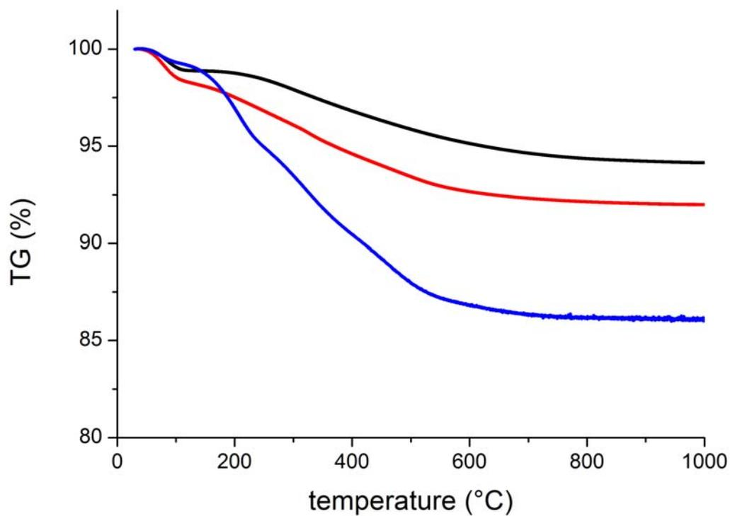
**Figure S6:** TGA curves of the bare particles ((1), black curve), the APTES covered particles ((2), red curve) and the CD covered particles ((4), blue curve).
