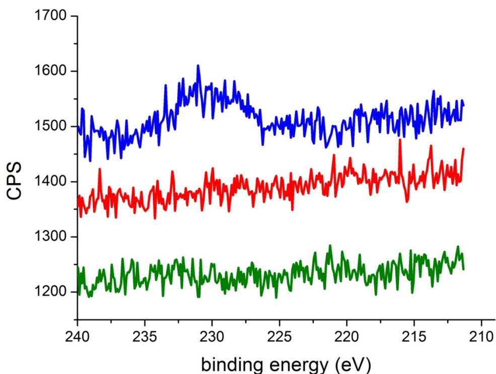
**Figure 5:** XPS narrow scan spectrum of the S1s signal of the bare particles ((1), green), the allyl particles ((3), red curve) and the CD covered particles ((5), blue curve).
