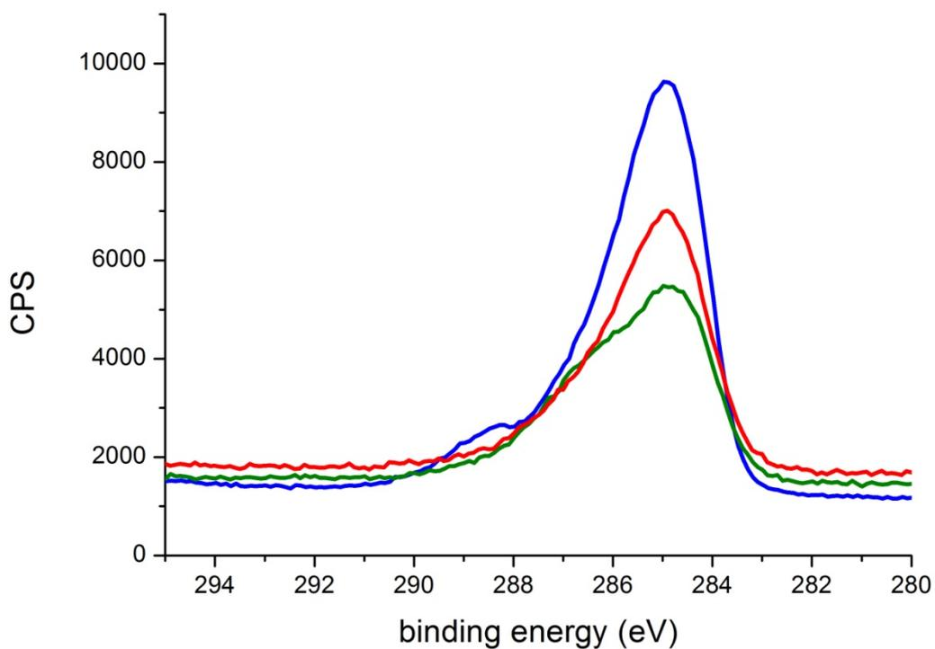
**Figure 4:** XPS narrow scan spectrum of the C1s signal of the bare particles ((1), green), the allyl particles ((3), red curve) and the CD covered particles ((5), blue curve).
