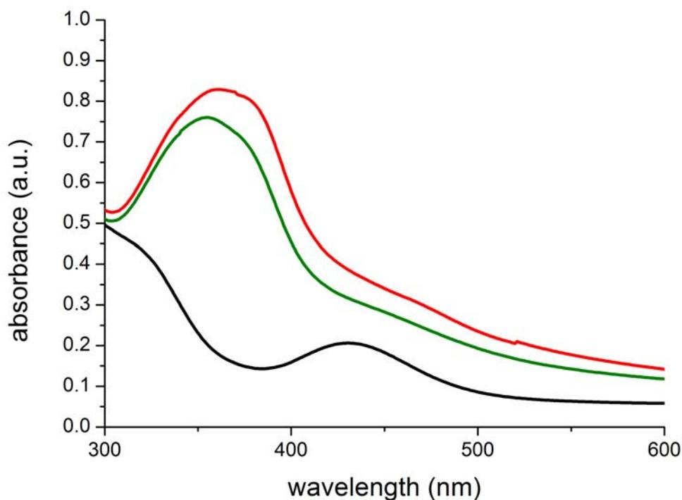
**Figure S10:** UV-vis spectra of  $\beta$ -CD-SH-NP (**5**) ( $c = 0.085$  mg/mL) in phosphate buffer after addition of the azobenzene linker (**6**) ( $c = 20\mu\text{M}$ ): Before (*trans*, red curve), after UV light irradiation ( $\lambda = 365$  nm) for 20 min (*cis*, black curve) and after visible light irradiation ( $\lambda = 455$  nm) for 20 min (*retrans*, green curve).
