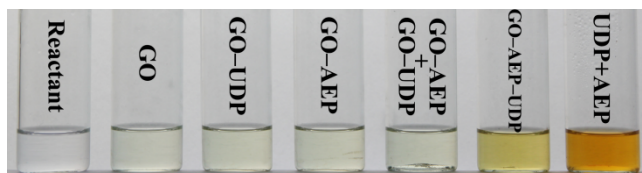
Fig. S4 photographs of product catalyzed by various catalysts. Product color is light yellow. The GO–AEP–UDP has the best performance. In the situation of homogeneous mixture comprising UDP and AEP, product color is orange, due to a great deal of byproducts.
