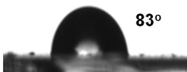
**Fig. S1** Static WCA for CNTs membrane after 30min UV irradiation.
