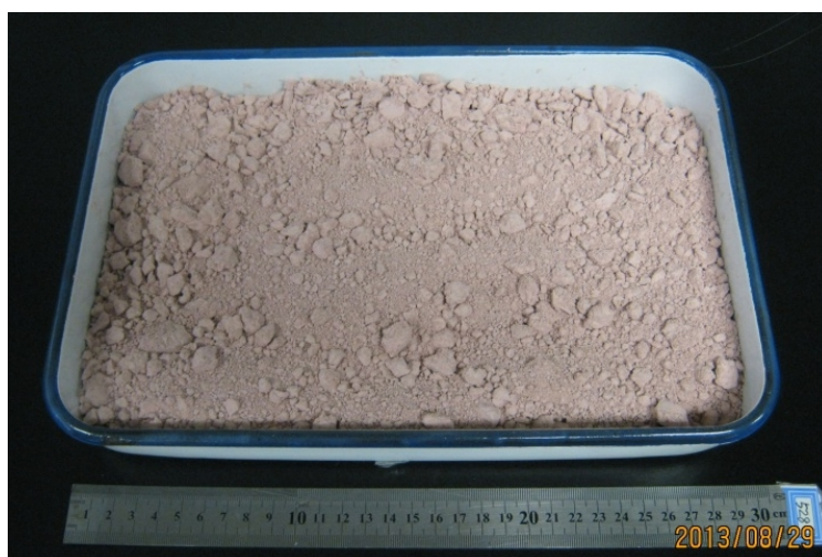
Figure S5. Photo of about 200 g of CoAl-LDH material from a scale up process.
