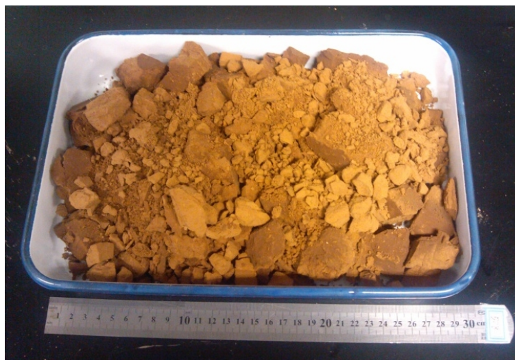
Figure S6. Photo of CoAl-LDH/Pd material (without the drying process) from a scale up process.
