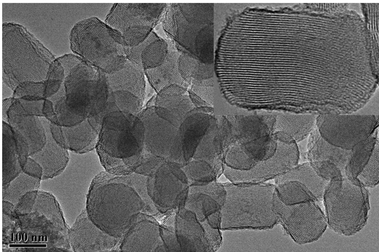
**Figure S5.** TEM image of rod-like MCM-41 with parallel channels along the long axis. The inset of TEM image with higher magnification shows ordered mesoporous structure with straight channels.
