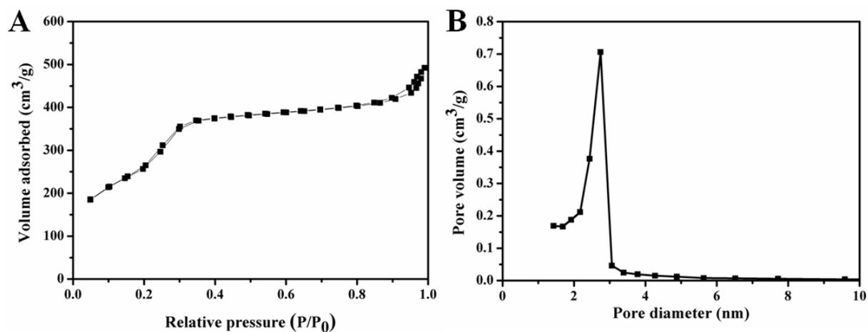
**Figure S4.** (A) N<sub>2</sub> adsorption-desorption isotherm of calcined ellipsoidal-like MCM-41; (B) The corresponding adsorption pore size distribution plot by BJH method.
