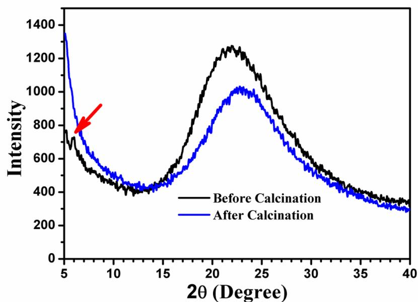
**Figure S3.** X-ray diffraction patterns of the ellipsoidal-like MCM-41 nanoparticles before and after calcination treatment.
