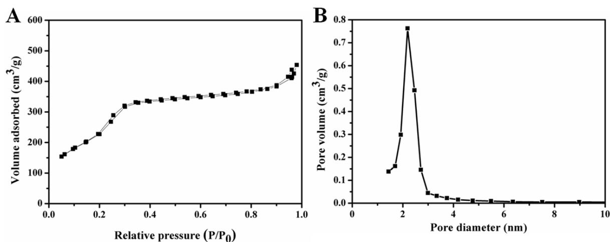
**Figure S7.** (A)  $\text{N}_2$  adsorption-desorption isotherm of ellipsoidal-like MCM-41 supported Ag nanocomposite; (B) The corresponding adsorption pore size distribution plot by BJH method.
