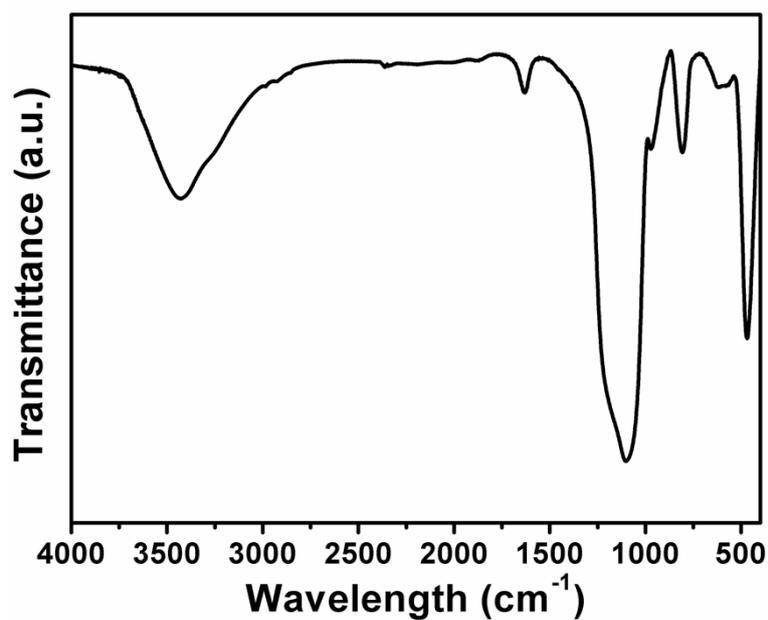
**Figure S2.** FT-IR spectra for the ellipsoidal-like MCM-41 nanoparticles after calcination treatment.
