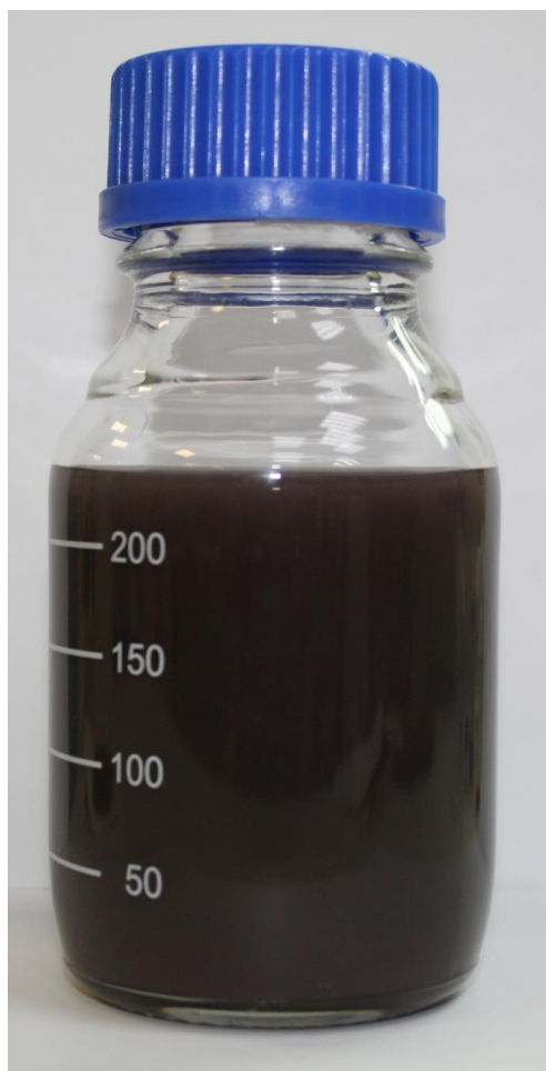
Figure S2. High yield of nanomaterials dispersion: Photograph of a high-quality dispersion of NbSe 2 in NMP (250 mL, 0.3 wt%).
