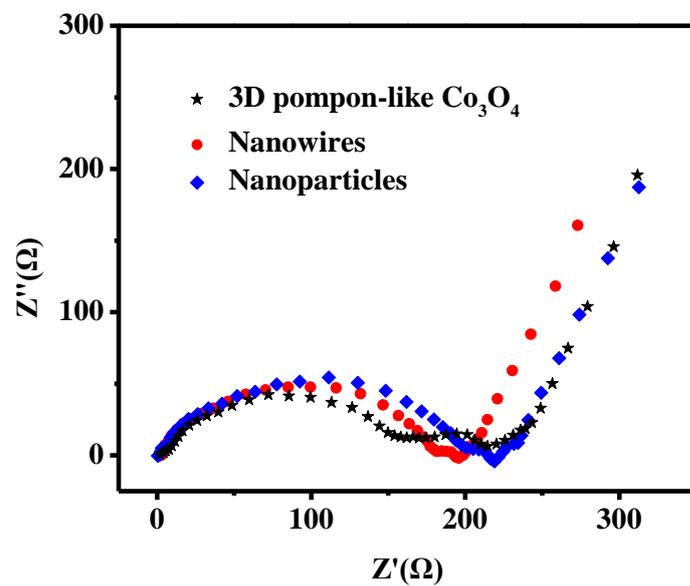
Fig. S5 Impedance spectra of three kinds of  $\text{Co}_3\text{O}_4$  at the 5th cycle.
