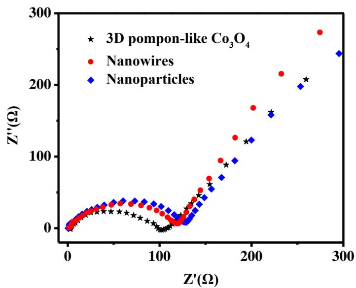
Fig. S4 Impedance spectra of three kinds of  $\text{Co}_3\text{O}_4$  before cycling
