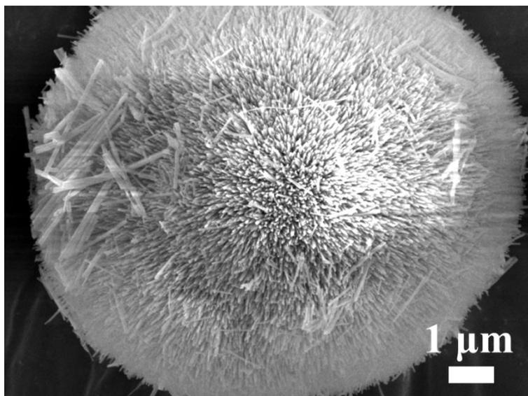
Fig. S3 SEM image of 3D pompon-like Co<sub>3</sub>O<sub>4</sub> after calcination
