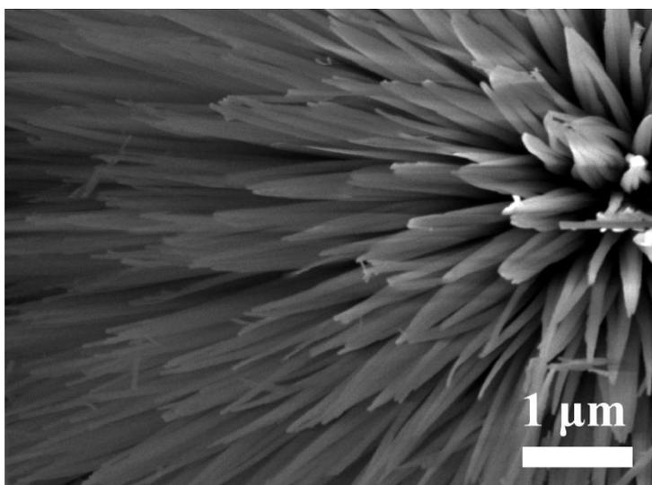
**Fig. S1** Specific SEM image of 3D pompon-like Co<sub>3</sub>O<sub>4</sub>
