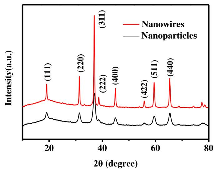
Fig. S2 XRD pattern of other two different kinds of Co<sub>3</sub>O<sub>4</sub> morphologies
