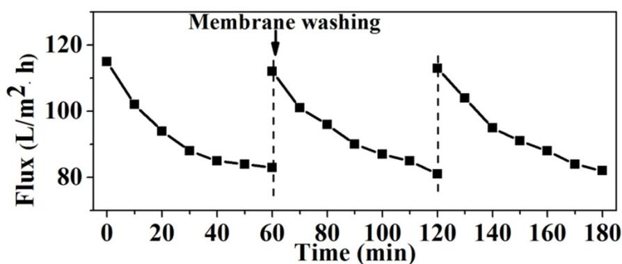
Figure S5 | The permeate flux of the membrane as the function of running time, and there is a membrane washing per 60 min to remove the oil residual.
