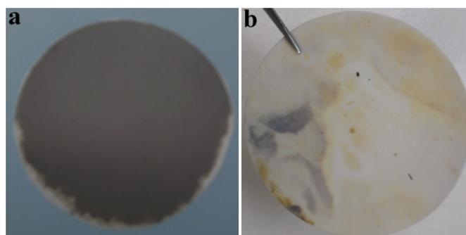
Figure S8 | Photos of graphene/TiO<sub>2</sub> membrane (a) and commercial PES membrane (b) after washing by water.
