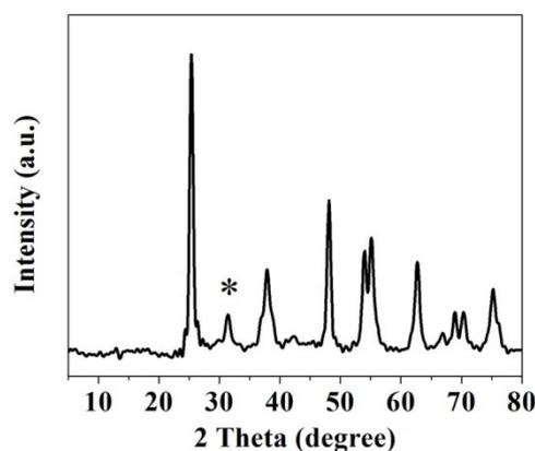
Figure S1 | XRD spectrum of SGO-TiO<sub>2</sub> membrane.
