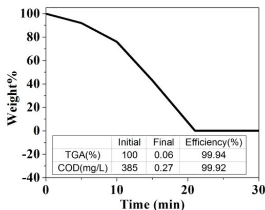
Figure S6 | TGA curve of crude oil-in-water emulsion after oil/water separation and COD results of crude oil-in-water emulsion before and after oil/water separation.
