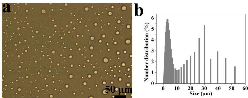
Figure S3 | (a) Optical microscopy images of toluene-in-water emulsions without surfactant showing the size of the oil droplets is in the range of 1-50 μm. (b) DLS data of toluene-in-water emulsions without surfactant confirming the size of the oil droplets is between 1 and 50 μm.
