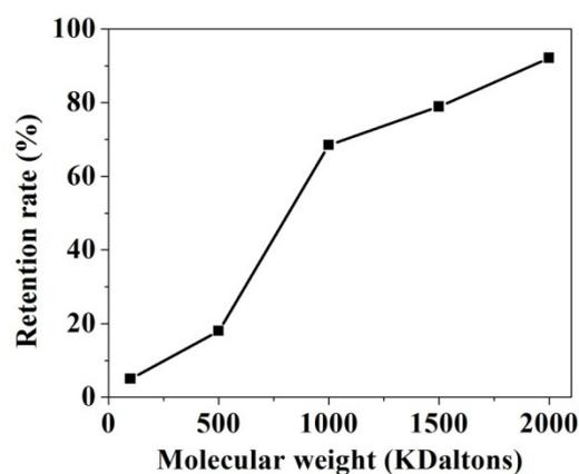
Figure S2 | Retention rates of dextran of different molecular weights by the SGO-TiO<sub>2</sub> membrane.
