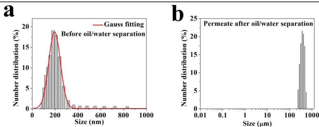
Figure S4 | (a) DLS data of the feed emulsions for surfactant-stabilized emulsions of toluene-in-water showing the oil droplet size is around 200 nm; (b) DLS data of the corresponding filtrate for surfactant-stabilized emulsions of toluene/water showing no oil droplets around these ranges are observed (the peak around 400 μm is an error signal caused by the machine).
