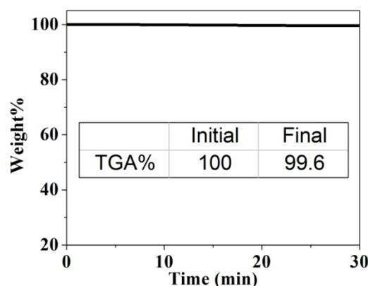
Figure S7 | TGA curve of separated crude oil after oil/water separation. Characterization of separated oil phase: Fig. S7 shows the TGA analysis of separated crude oil after oil/water separation. The TGA results indicate that the majority part of the separated oil phase is crude oil, and only around 0.4% is water, which can be attributed to the superhydrophilic and superoleophobic properties of the membrane.
