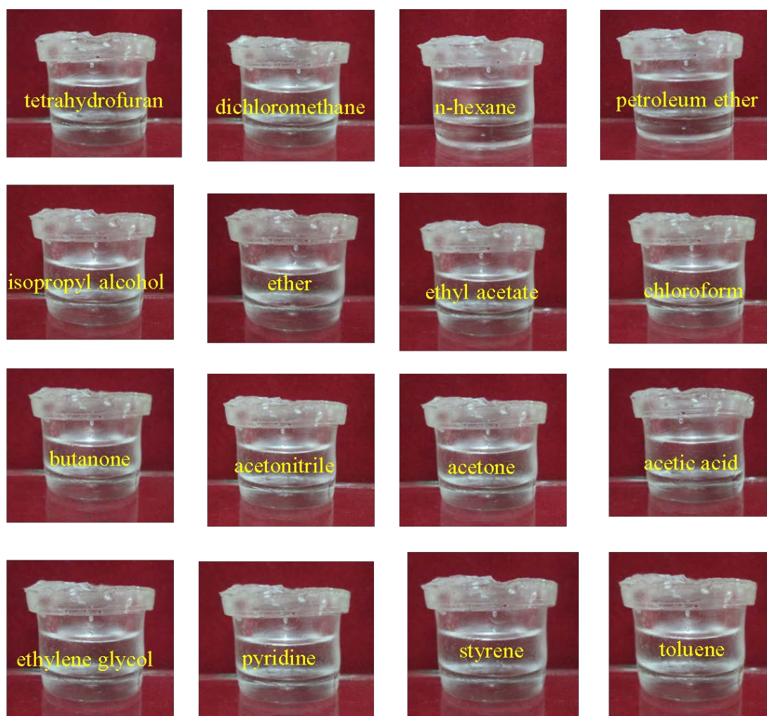
Figure S5. A PAMPSA cup filled with common organic solvents. No damage to the cup is observed after filling with organic solvents and waiting for 30 min, indicating that the PAMPSA material has good chemical resistance.
