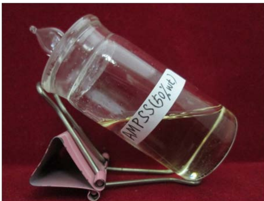
Figure S3. No hydrogel formed from the 2-acrylamido-2-methyl-1-propanesulfonic sodium (AMPSS) aqueous solution (50 wt%) after heating at 80 °C for 2 h, indicating that the high polymerization activity of AMPSA might be due to the catalytic effect of the counterion H^+ of the sulfonic group. Here, AMPSS was prepared from AMPSA by cation exchange resin.
