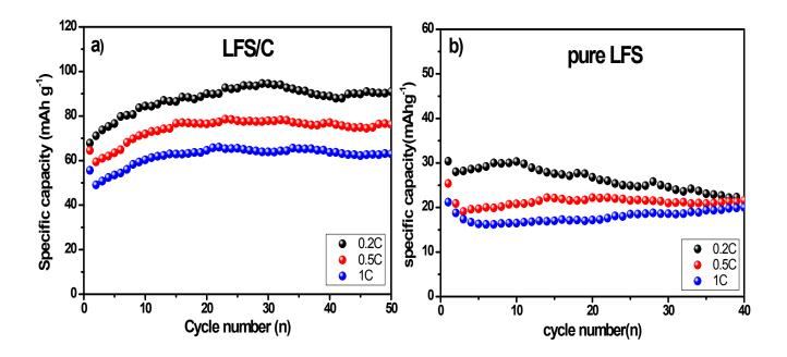
**Fig.S2** Cycling performances of LFS-3d with a) and without b) carbon coating at various current densities.
