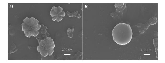
Fig.S3 SEM images of LFS/C-3d hollow sphere cathode after 50 cycles under 1C rate.
