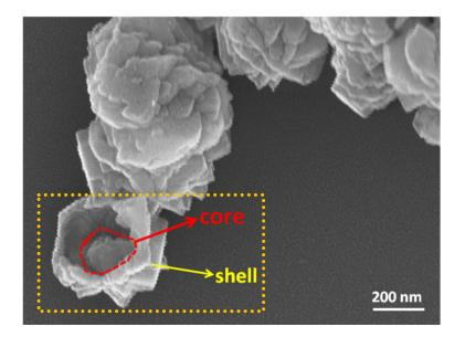
Fig.S1 SEM image of LFS hydrothermal synthesized for two days which obviously shows a core-shell structure.
