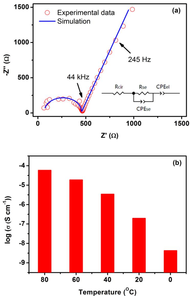
**Fig. S2** (a) Electrochemical impedance spectroscopy (EIS) profile of the dry polymer electrolyte at 80 °C. The inset shows the equivalent circuit utilized for simulation. (b) The conductivities of the dry polymer electrolyte at different temperature.
