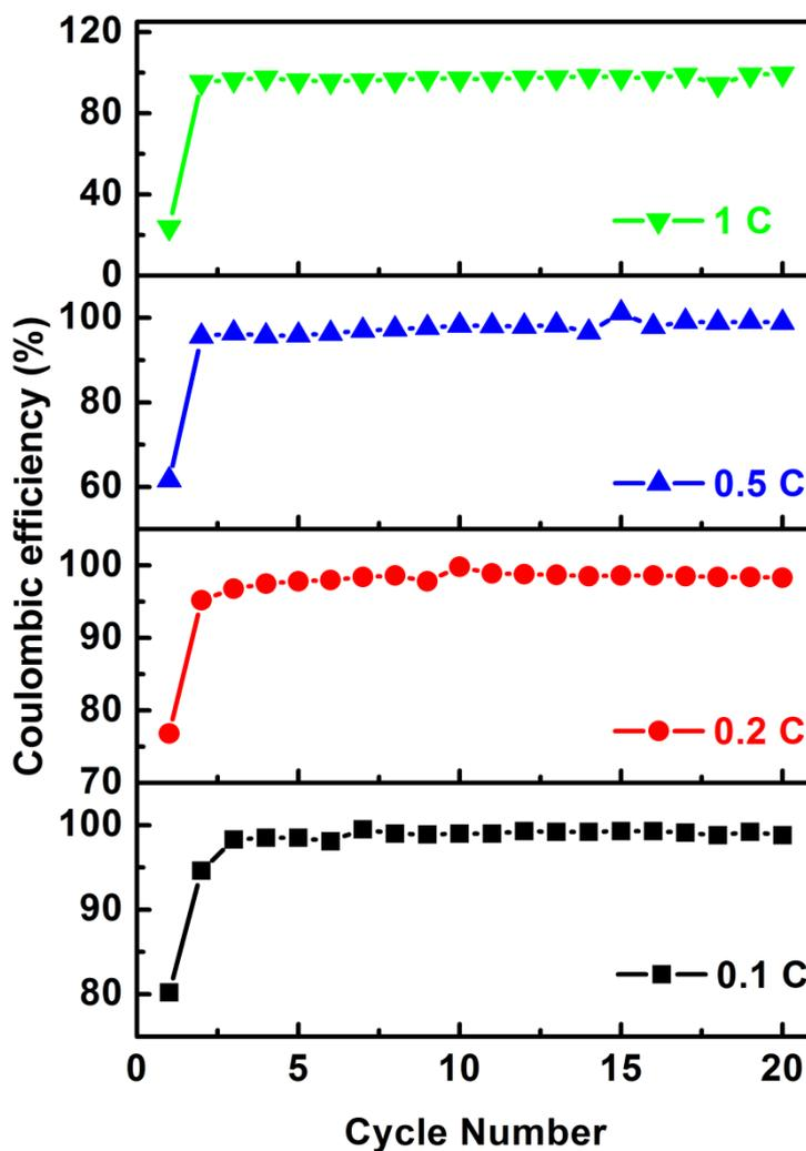
**Fig. S1** The Coulombic efficiency of the 811 composite electrodes at various discharge current rates.
