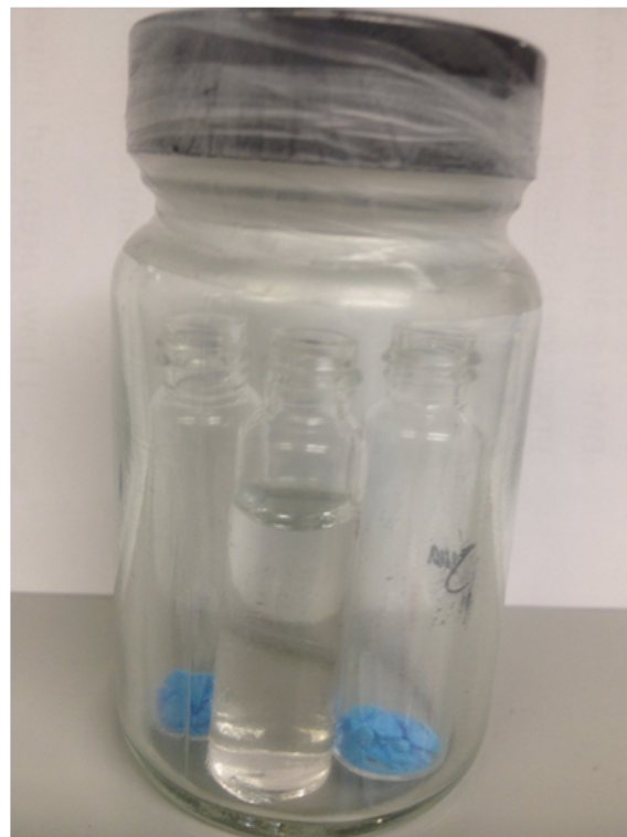
Figure S9. Experimental set-up to control the moisture exposure to C_n Gua-HKUST-1 phases when investigating the role of water in the etching process. (Left) samples were placed in a desiccator to provide a low humidity environment relative to the laboratory atmosphere and (right) a sealed vessel containing C_n Gua-HKUST-1 and an open vial of water to increase humidity levels.
