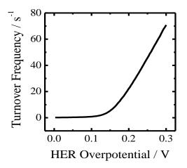
**Figure S3**. Turnover frequency of cobalt selenide films as function of overpotential for the hydrogen-evolution reaction in 0.500 M  $H_2SO_4$  saturated with  $H_2(g)$  derived from the voltammetric data in Figure 2a.
