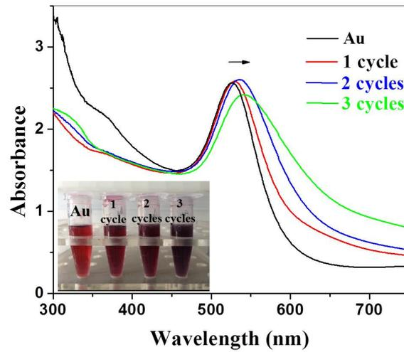
**Fig. S2** UV-vis spectra of bare Au NPs, Au@TA-Fe composites with 1, 2, and 3 assembly cycles. The inset shows the color of the corresponding solution.
