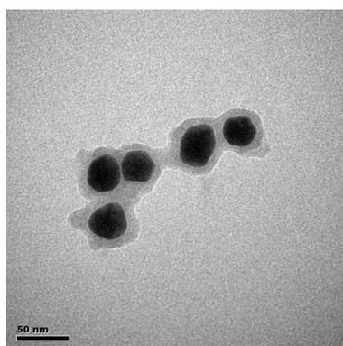
**Fig. S7** TEM image of Au@TA-Fe nanocatalyst after used.
