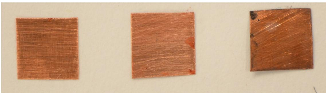
**Figure S2.** The corresponding optical image of the other side of Cu discs at each step of treatment showing that no  $\text{Fe}_2\text{O}_3/\text{C}$  layer or  $\text{Fe}_3\text{O}_4/\text{C}$  layer coated on the other side of copper discs: from the left to the right, back view of bare  $\rightarrow$   $\text{Fe}_2\text{O}_3/\text{C}$  layer coated  $\rightarrow$   $\text{Fe}_3\text{O}_4/\text{C}$  layer coated Cu discs.
