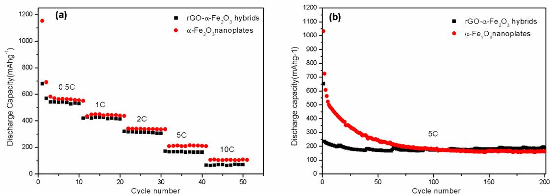
**Figure S8.** Rate performance (a) and cycling performance at 5C rate (b) of the samples prepared without adding of glycerol or graphene oxide
