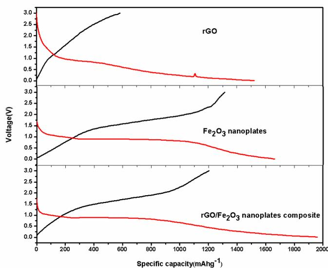
**Figure S7.** The representative charge-discharge curves of the rGO,  $\alpha$ -Fe<sub>2</sub>O<sub>3</sub> nanoplates and rGO/ $\alpha$ -Fe<sub>2</sub>O<sub>3</sub> nanoplate composite for the first cycle.
