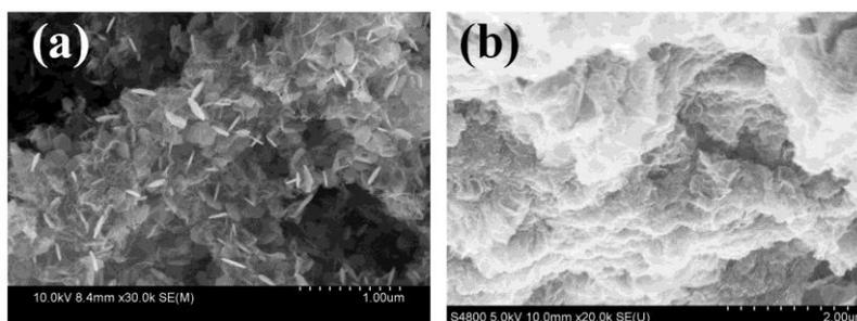
**Figure S3.** SEM images of (a) the rGO/ $\alpha$ -Fe<sub>2</sub>O<sub>3</sub> nanoplate composite and (b) rGO without adding FeSO<sub>4</sub> · 7H<sub>2</sub>O
