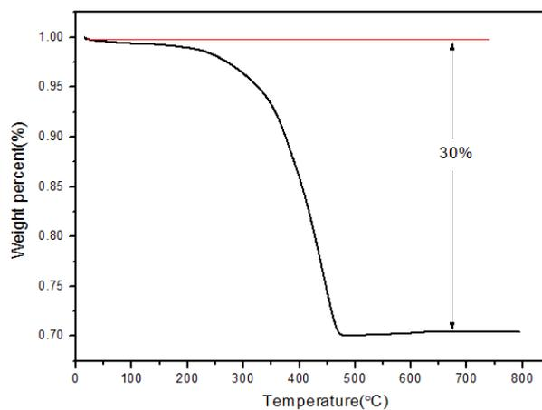
**Figure S6.** TG curves of the samples prepared at 180°C
