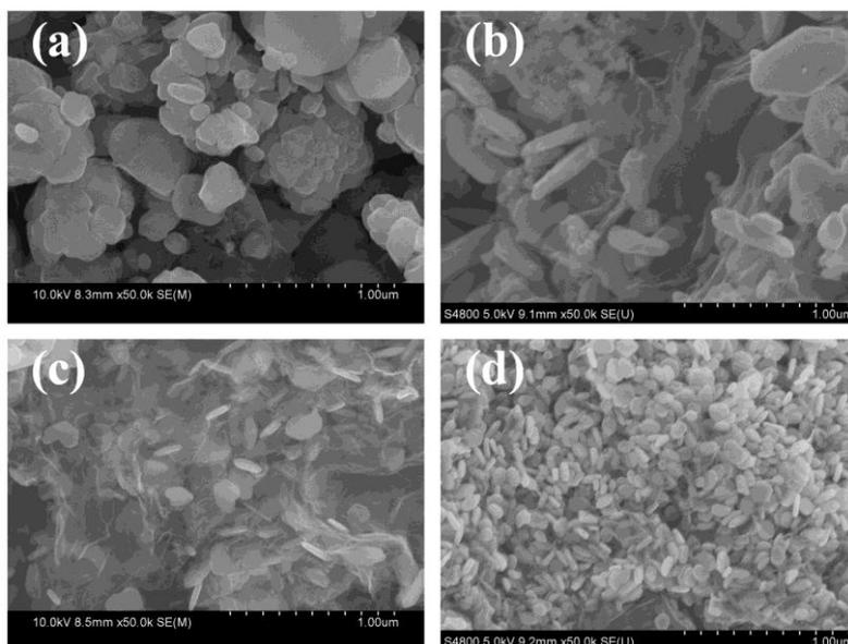
**Figure S5.** SEM images of the samples prepared with different amount of glycerol (a) 0ml, (b) 10ml, (c) 20ml, (d) 40ml while the total amount of the solvent kept unchanged
