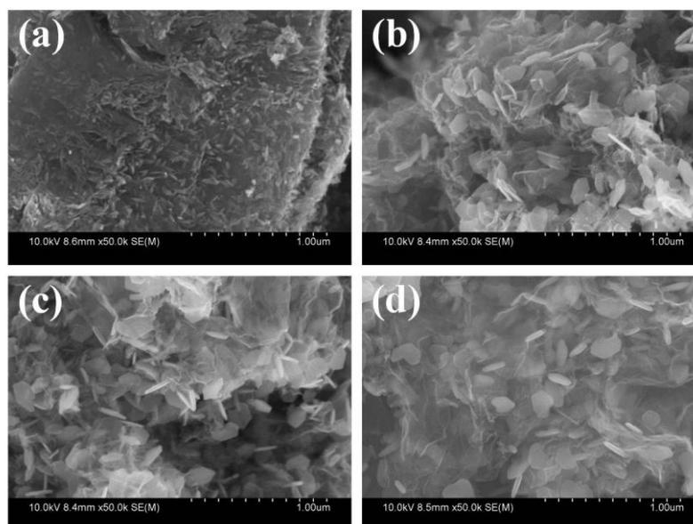
**Figure S1.** SEM images of the samples prepared under different temperature: (a)120°C; (b) 140°C; (c) at 160°C; (d)180°C.
