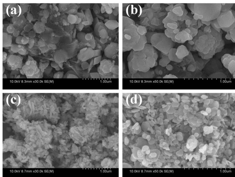
**Figure S4.** SEM images of the samples prepared without adding of glycerol (a) (b) and without adding of graphene oxide (c) (d)
