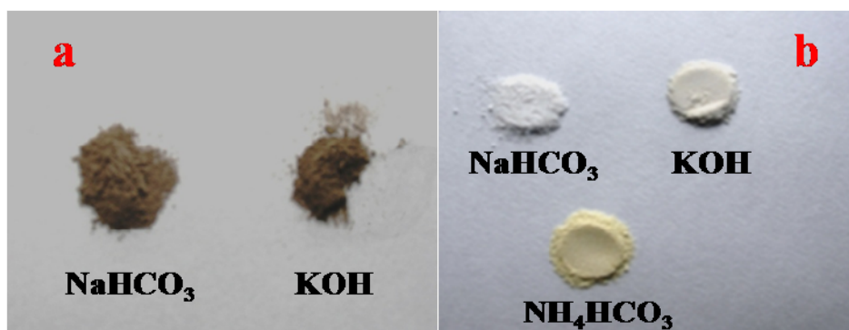
Figure S2. (a) A photo of \text{TiO}_2 heated at 200^\circ\text{C} that synthesized from \text{NaHCO}_3 and \text{KOH} respectively; (b) A photo of \text{TiO}_2 heated at 400^\circ\text{C} that synthesized from \text{NaHCO}_3 , \text{KOH} and \text{NH}_4\text{HCO}_3 respectively. The contrast experiments confirmed that the hydroxylation induced the brown colour and the N-doping induced the yellow colour.
