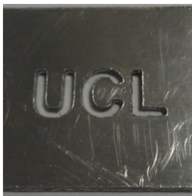
Photograph of the CNC-milled aluminum 'UCL' lettering cut-out template.
