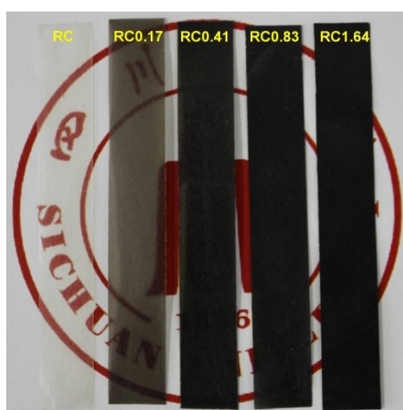
Fig. S1 Optical image of ~0.09 mm-thick GONS/cellulose nanocomposite films as a function of GONS loadings.
