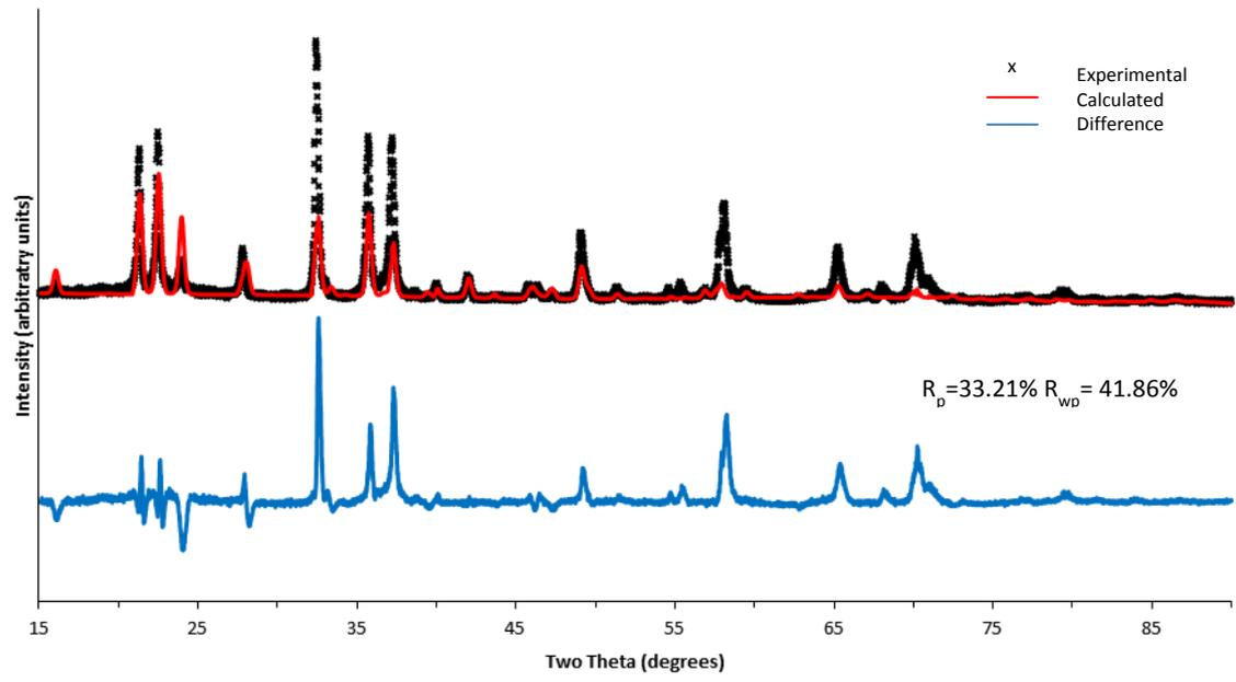
**Figure S2. X-ray diffraction pattern comparison of hydro-LCG to simulated diffraction patterns of different LCG polymorphs from 15-90 ° two theta.**
