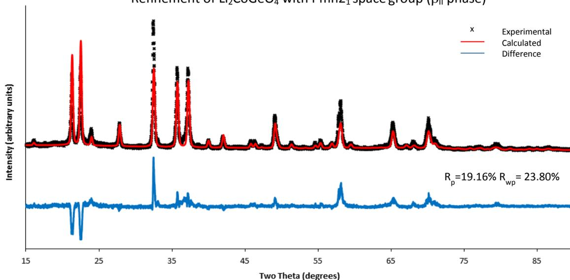
Refinement of  $\text{Li}_2\text{CoGeO}_4$  with  $P2_1/n$  space group ( $\gamma_0$  phase)
