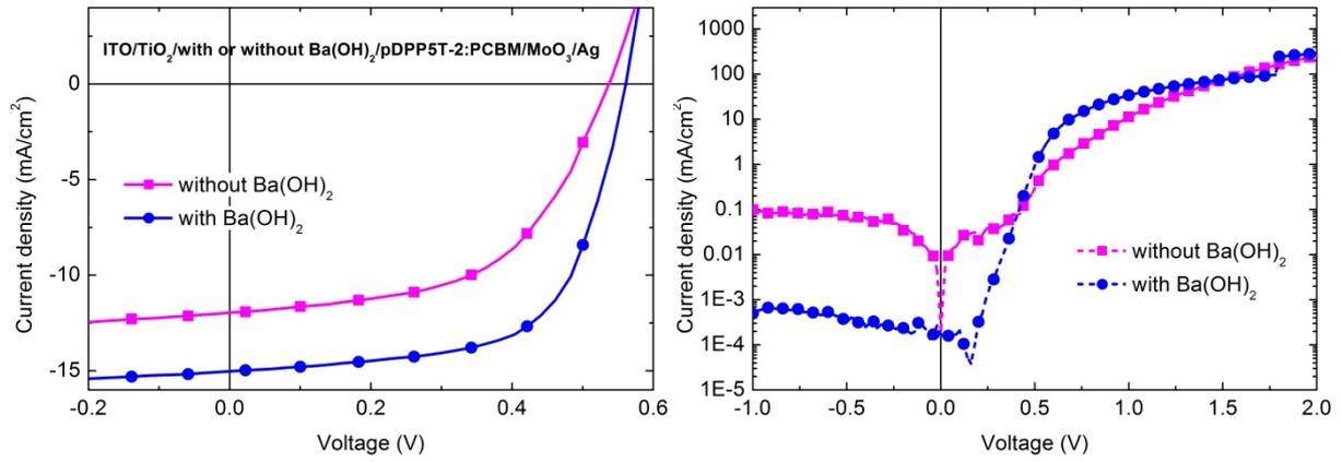
Figure S3. a)  $j$ - $V$  characteristics of inverted pDPP5T-2:PC<sub>61</sub>BM organic solar cells without and with the Ba(OH)<sub>2</sub> layer on TiO<sub>2</sub> layer. b) Corresponding logarithmic plot of dark  $j$ - $V$  characteristics.
