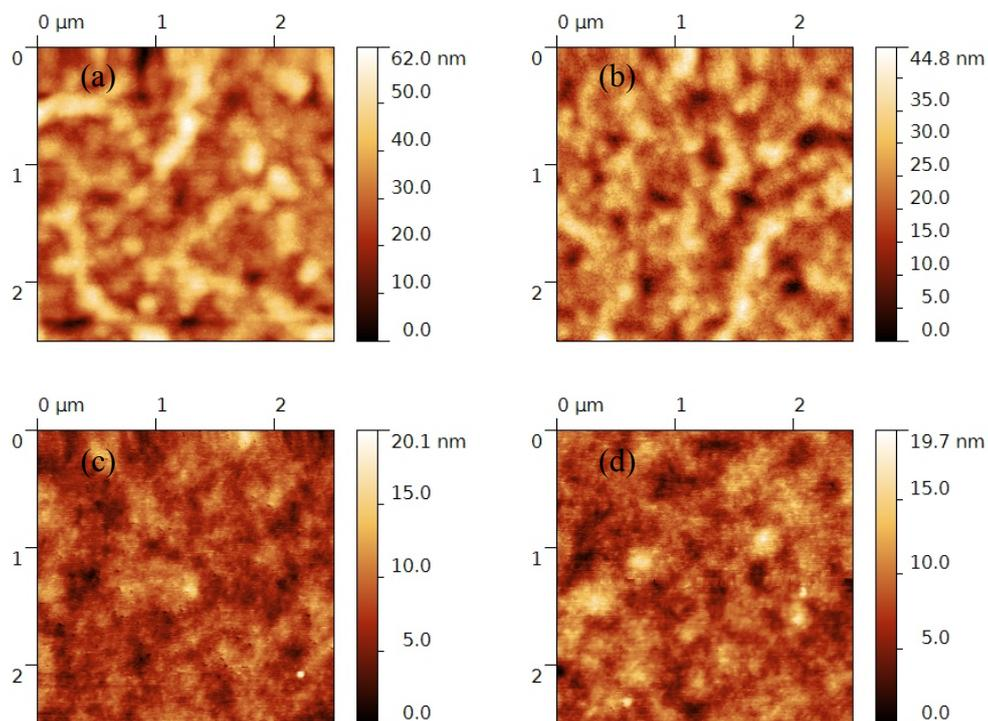
Figure S4. Surface topographic AFM images (size:  $2.5 \times 2.5 \mu\text{m}^2$ ) of (a) bare AZO layer, (b) thin  $\text{Ba}(\text{OH})_2$  on the AZO layer, (c) pDPP5T-2:PC<sub>61</sub>BM BHJ film on the AZO layer without  $\text{Ba}(\text{OH})_2$  inserted and (d) (c) pDPP5T-2:PC<sub>61</sub>BM BHJ film on the AZO layer with  $\text{Ba}(\text{OH})_2$  inserted.
