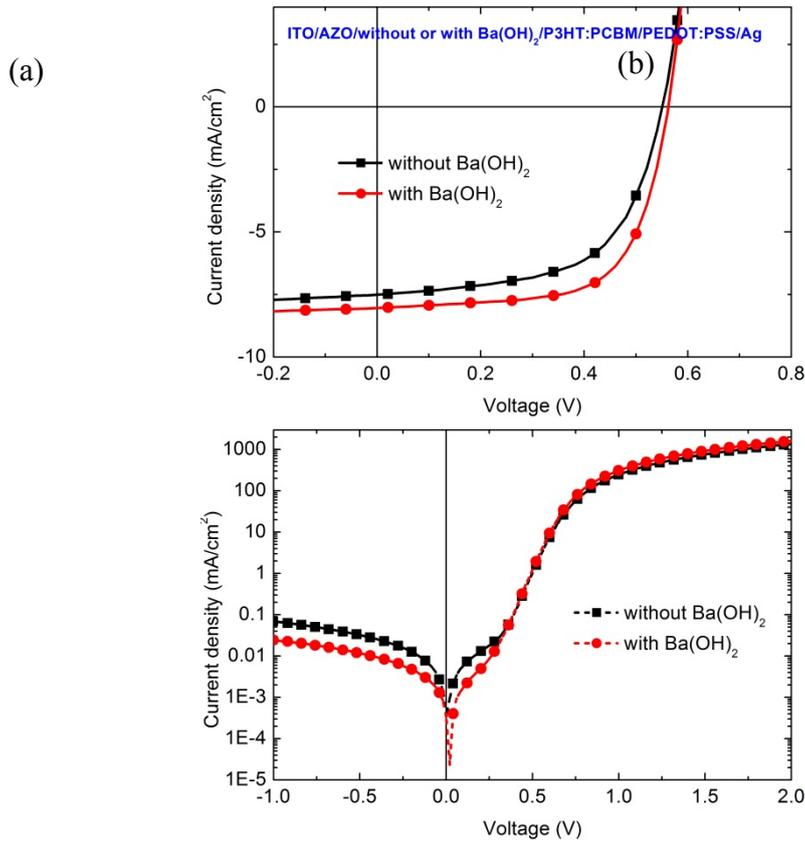
Figure S7. a)  $j$ - $V$  characteristics of inverted P3HT:PC<sub>61</sub>BM organic solar cells without and with the Ba(OH)<sub>2</sub> layer. b) Corresponding logarithmic plot of dark  $j$ - $V$  characteristics.
