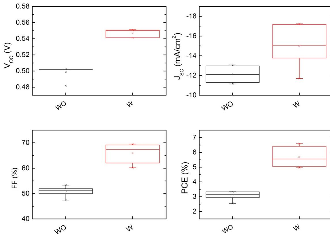
Figure S2. Photovoltaic parameters distribution of over 6 solar cells; the boxes represent the 25–75% distribution range, and hollow squares represent the mean values (WO = without Ba(OH)<sub>2</sub> and W = with Ba(OH)<sub>2</sub>).
