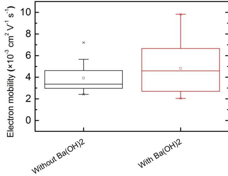
Figure S6. The box chats is obtained from  $j$ - $V$  fitting on 12 electron-only devices without and with the Ba(OH)<sub>2</sub> layer.
