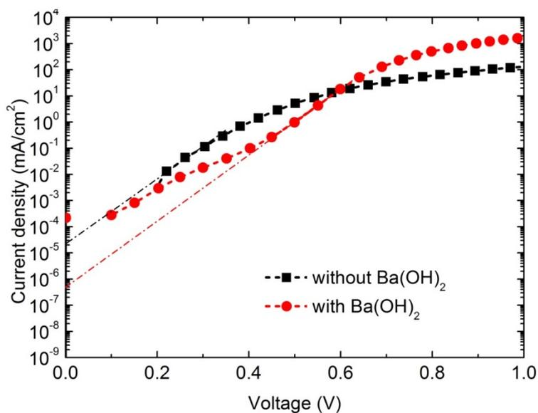
Figure S5. Semilog plot of dark  $j$ - $V$  characteristics curves of inverted organic solar cells without and with the  $\text{Ba}(\text{OH})_2$  layer. The dashed lines show the extrapolated line for determining saturation current density from intercept and diode ideality factor from the slope.
