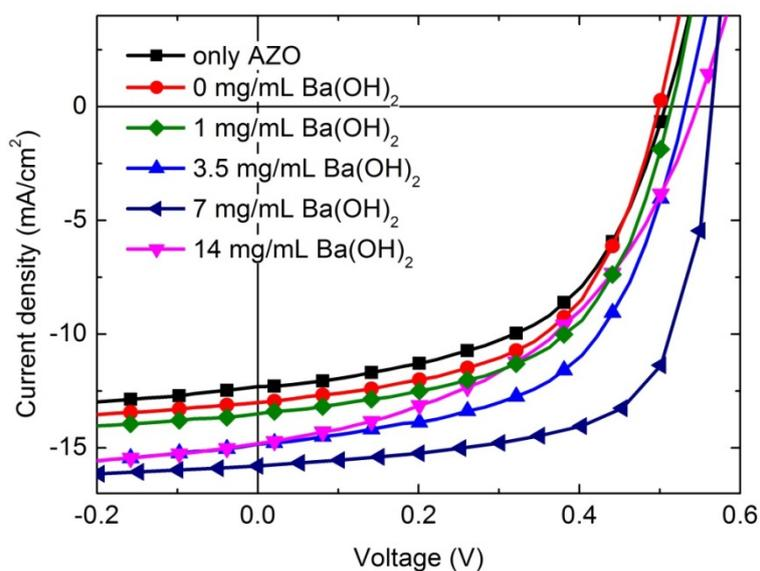
Figure S1.  $j$ - $V$  characteristics of typical devices with different concentrations of  $\text{Ba}(\text{OH})_2$ .
