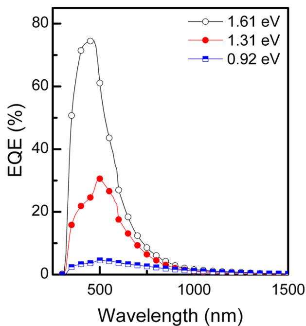
Fig. S1 Absolute EQE spectra of the photovoltaic cells for the PbS thin films with different band gaps.
