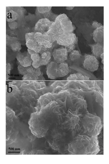
Figure S2 shows SEM and TEM images of NiS nanoparticles prepared from L-cysteine instead of thiourea.
