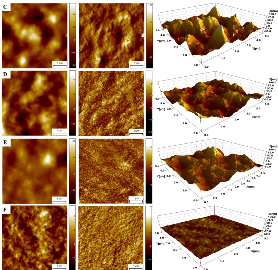
**Figure ESI 1.** AFM topography, corresponding phase images (5  $\mu\text{m} \times 5 \mu\text{m}$ ) and 3D surface representation of the annealed samples of P3HT:PCBM blends processed without (A) and with additives: CN 3% (B), CN 5% (C), NMP 3% (D), NMP 5% (E), BARB 1% (F). The scale bars are 1  $\mu\text{m}$ . 3D representation has a fix orientation and axis scale (max.100 nm; min.-50 nm) for comparison purposes.
