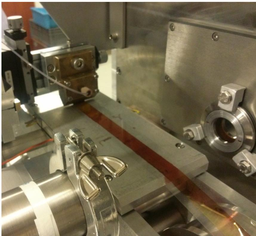
**Figure ESI 4.** Schematic representation and a corresponding picture of the slot-die coating device incorporated to SAXS instrument allowing control of the pump rate, speed and temperature of the film deposition. The solvent evaporation time was modified by varying the distance between the coating position versus the X-ray beam.
