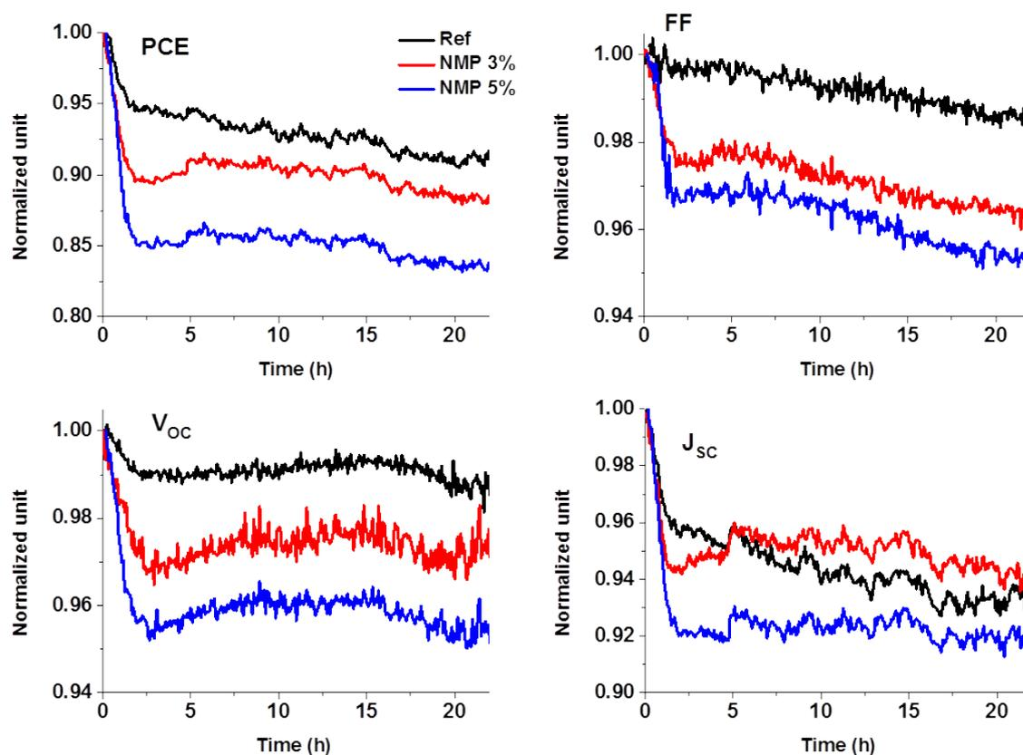
**Figure ESI 7.** Representative examples of degradation curves for devices fabricated with CN, BARB and NMP with the best performing device architectures; “3 layer” for CN and BARB, “5010” for NMP. The normalized PCE, FF, Voc and Jsc are plotted over time; curves of the reference tested concomitantly with the samples are presented for comparison.
