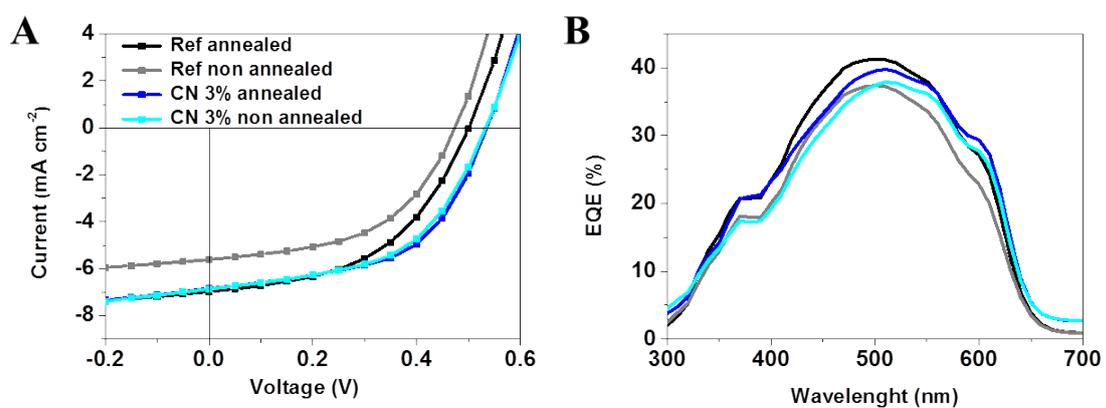
**Figure ESI 6.** J-V curves (A) and EQE spectra (B) of the annealed and non-annealed devices (area of 1 cm<sup>2</sup>) coated without and with the 3% CN additive.
