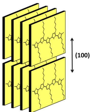
**Figure ESI 2.** Schematic representation of P3HT crystalline edge-on orientation and lamellar spacing at  $100$  reflection.
