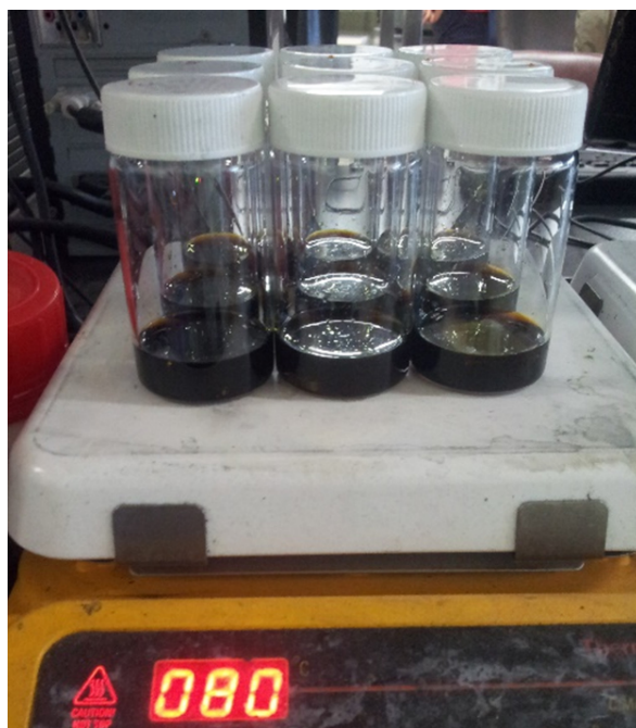
Figure S5. Stability test of the as-prepared bipolar plates in vanadium electrolyte solution at 80 °C for a week.
