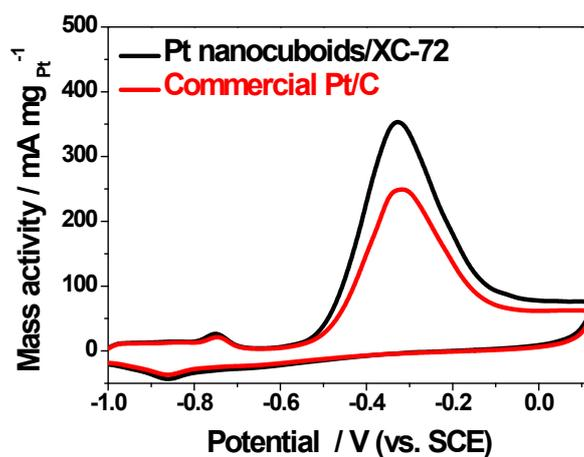
**Fig. S11** Cyclic voltammograms for 20 wt.% Pt nanocuboids/XC-72 and 20 wt.% commercial Pt/C in N<sub>2</sub>-saturated 1 M KOH + 0.1 M NH<sub>4</sub>OH solution at the scan rate of 10 mV s<sup>-1</sup>. For the preparation of 20% wt.% Pt nanocuboids/XC-72 catalyst, 4 mg of Vulcan XC-72 carbon black was added into 10 mL of 0.1 mg mL<sup>-1</sup> Pt nanocuboids suspension with continued stirring for 2 h.
