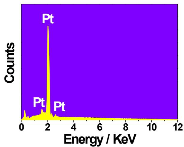
Fig. S1 EDX spectrum of the as-prepared Pt nanocuboids.
