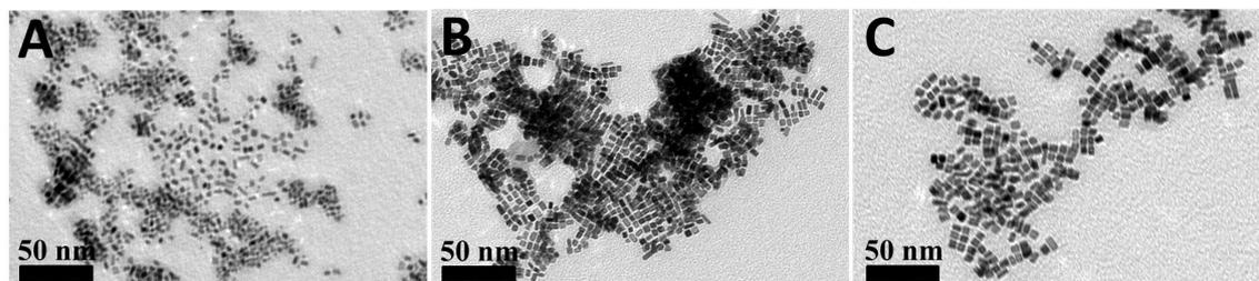
**Fig. S9** TEM images of Pt nanocrystals prepared at different reaction times: (A) 140 °C, (B) 160 °C and (C) 180 °C.
