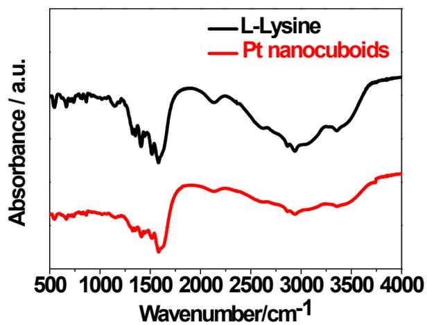
**Fig. S6** FT-IR spectra of as-prepared Pt nanocuboids and L-Lysine.
