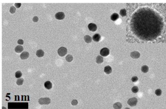
**Fig. S7** TEM image of Pt nanocrystals prepared by displacing the air with O<sub>2</sub>.
