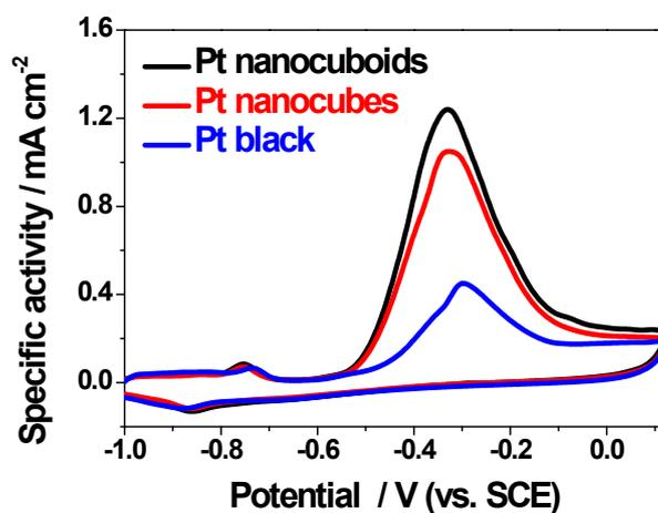
**Fig. S12** Cyclic voltammograms for Pt nanocuboids, Pt nanocubes and Pt black in N<sub>2</sub>-saturated 1 M KOH + 0.1 M NH<sub>4</sub>OH solution at the scan rate of 10 mV s<sup>-1</sup>, 5 nm Pt nanocubes were synthesized under the same conditions as in Fig. 3B.
