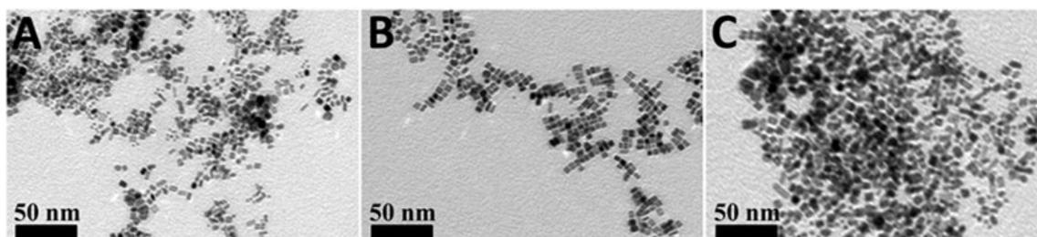
**Fig. S8** TEM images of Pt nanocrystals prepared at different Pt<sup>II</sup> precursor volumes: (A) 0.5 ml, (B) 1.0 ml and (C) 4.0 ml.
