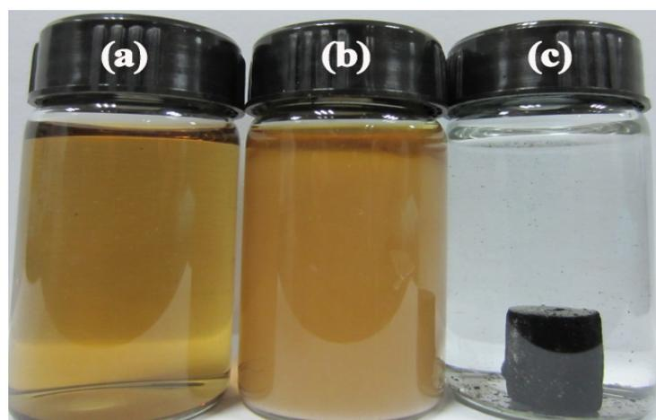
**Figure S2.** Optical image of (a) GO suspension, (b) suspension of TiO<sub>2</sub> and GO before hydrothermal treatment, and (c) the TiO<sub>2</sub>-rGO composite after hydrothermal treatment at 180°C for 12 h.
