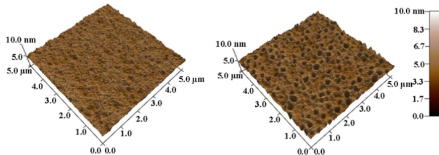
**Figure S2.** 3D images obtained by tapping-mode AFM of ASQ:PC<sub>71</sub>BM (1:8, w/w) composite films. Left: **1a**, Right: **1b**.
