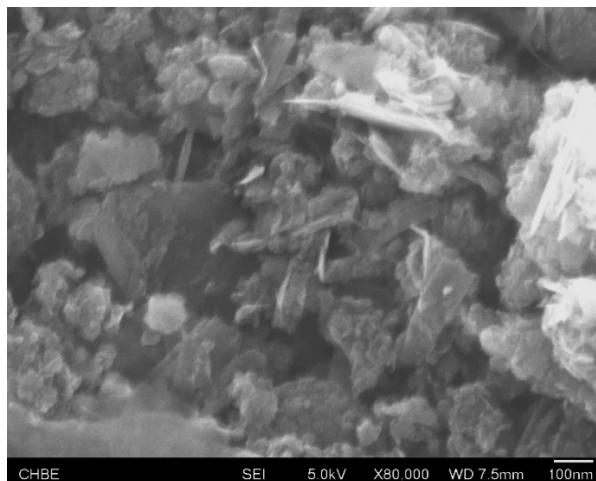
**Figure S3.** FESEM characterization of pure GNP membrane.
