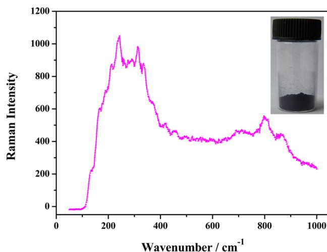
Fig. S3 Raman spectrum of the W<sub>18</sub>O<sub>49</sub> nanowire arrays.
