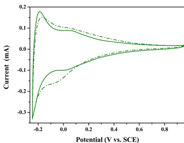
**Fig. S7** ADT recorded in an Ar-purged 0.5 M H<sub>2</sub>SO<sub>4</sub> with a sweep rate of 100 mV·s<sup>-1</sup> of the W<sub>18</sub>O<sub>49</sub> NRs support (solid for the 1<sup>st</sup> cycle and dotted for the 5000<sup>th</sup> cycle).
