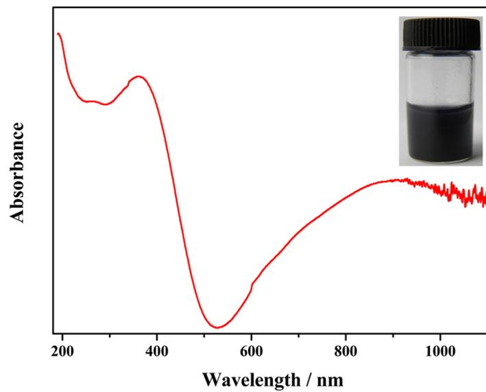
**Fig. S5** Ultraviolet/visible (UV/Vis) absorption spectrum of the  $W_{18}O_{49}$  NRs.
