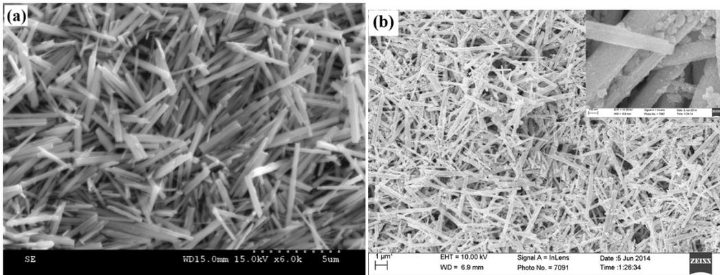
**Fig. S4** SEM image of the (a)  $W_{18}O_{49}$  NRs and (b) Pt/ $W_{18}O_{49}$ . High-magnification SEM image of Pt/ $W_{18}O_{49}$  is shown in the inset of (b).
