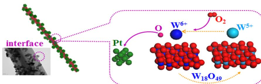
Fig. S2 Mechanism of the oxygen buffering effect in Pt/W<sub>18</sub>O<sub>49</sub>.
