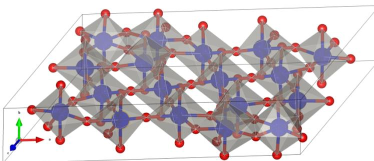
Fig. S1 Crystal structure of the monoclinic W<sub>18</sub>O<sub>49</sub>.
