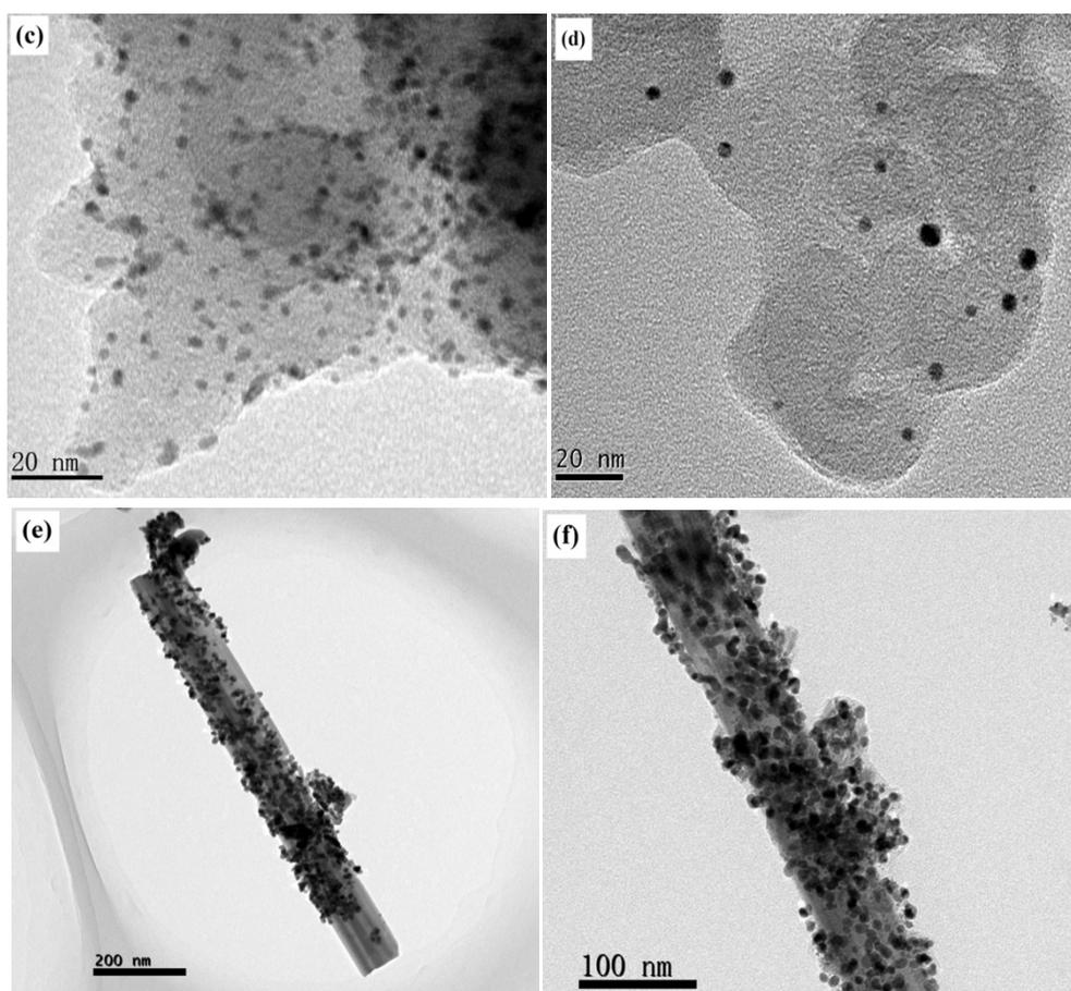
**Fig. S6** TEM images of Pt-black: (a) dispersion before the durability test and (b) aggregation/Oswald ripening after a 5000-cycle durability test. Pt/C: (c) dispersion before the durability test and (d) dissolution/aggregation/Oswald ripening after a 5000-cycle durability test. Pt/W<sub>18</sub>O<sub>49</sub>: (e) dispersion before the durability test and (f) dispersion almost unchanged after a 5000-cycle durability test.
