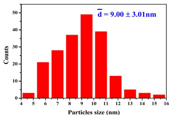
**Fig. S8** The corresponding particle size distribution obtained by counting 200 Pt particles of Pt/W<sub>18</sub>O<sub>49</sub> after a 5000-cycle ADT in Fig. S6f.
