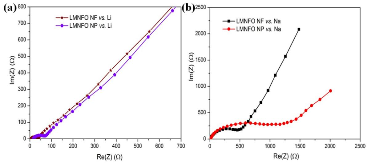
**Fig. S6:** Electrochemical impedance spectroscopy Nyquist plots of LMNFO NF and LMNFO NP in (a) LIBs and (b) SIBs, at open circuit voltage and in the frequency range of 100 kHz to 100 mHz.
