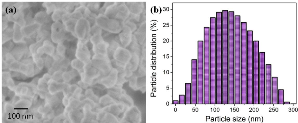
**Fig. S1:** (a) SEM image of LMNFO NP and (b) corresponding particle size distribution.
