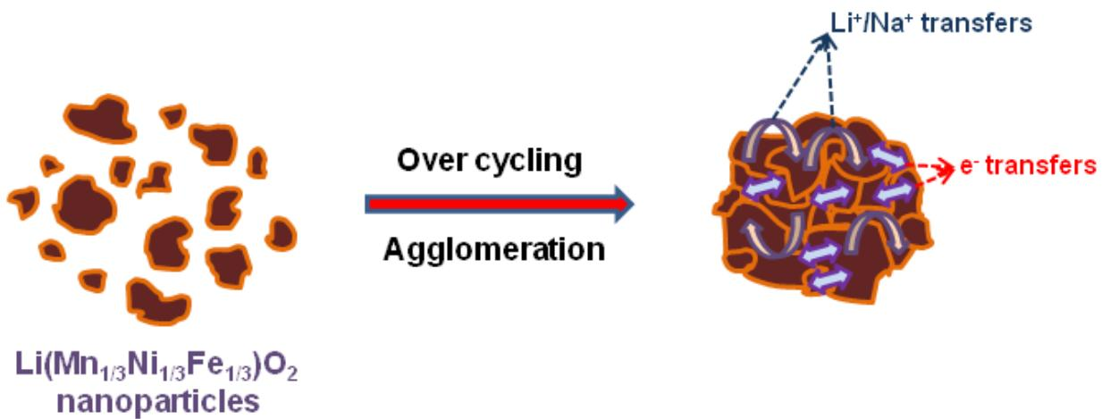
**Fig. S5:** Schematic representation of the self-agglomeration phenomenon in nanoparticles that occur during cycling and their charge transfer kinetics.
