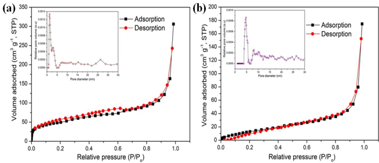
**Fig. S2:** N<sub>2</sub> adsorption and desorption isotherms of (a) LMNFO NF and (b) LMNFO NP (insets: pore diameter size distribution of LMNFO NF and LMNFO NP, respectively).
