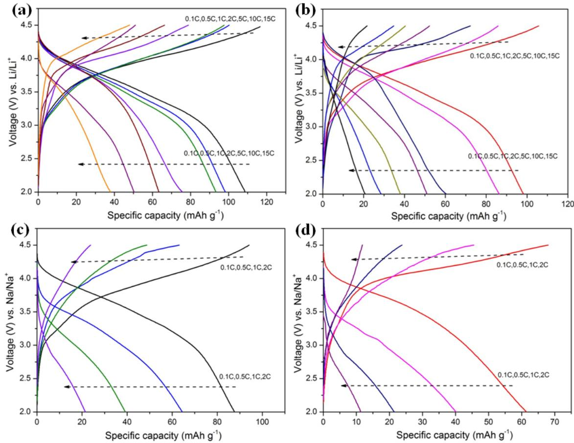
**Fig. S4:** (a) & (b) Charge-discharge curves of LMNFO NF and LMNFO NP, respectively at various current rates in LIBs; (c) & (d) Charge-discharge curves of LMNFO NF and LMNFO NP, respectively, at various current rates in SIBs, in the voltage range of 2 – 4.5 V.
