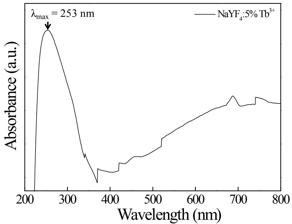
**Figure S2:** UV-visible absorption spectra of  $\beta$ -NaYF<sub>4</sub>:5 % Tb<sup>3+</sup>.
