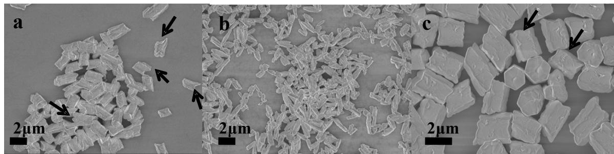
**Figure S1.A:** FESEM imaged of  $\beta\text{-NaYF}_4\text{:5 \% Tb}^{3+}$  crystals prepared using only (a) trisodium citrate, (b) only CTAB and (c) trisodium citrate together with CTAB.
