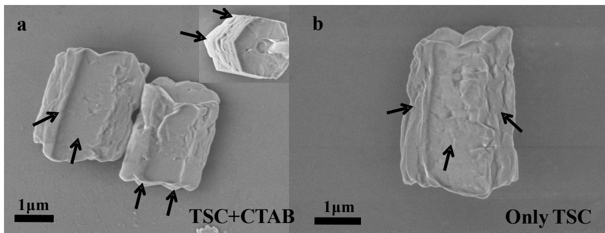
**Figure S1.B:** Magnified FESEM images of  $\beta\text{-NaYF}_4\text{:5 \% Tb}^{3+}$  crystals prepared using (a) trisodium citrate and CTAB both and (b) only trisodium citrate. Arrows indicating well define, smooth and sharp edges of prismatic side planes formed in presence of both trisodium citrate and CTAB in converse to relatively less smooth and sharp prismatic side plane, when prepared using only trisodium citrate.
