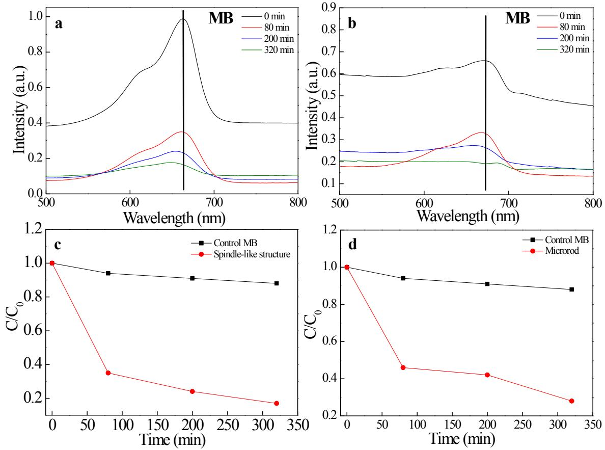
**Figure S4:** Photocatalytic degradation of MB in presence of  $\beta\text{-NaYF}_4\text{:5 \% Tb}^{3+}$  with (a) spindle-like structure, and (b) microrods under irradiation of 400 W mercury lamp for 320 min. Plots of dye concentrations ( $C/C_0$ ) vs. time for (c) spindle-like structure and (d) microrods.
