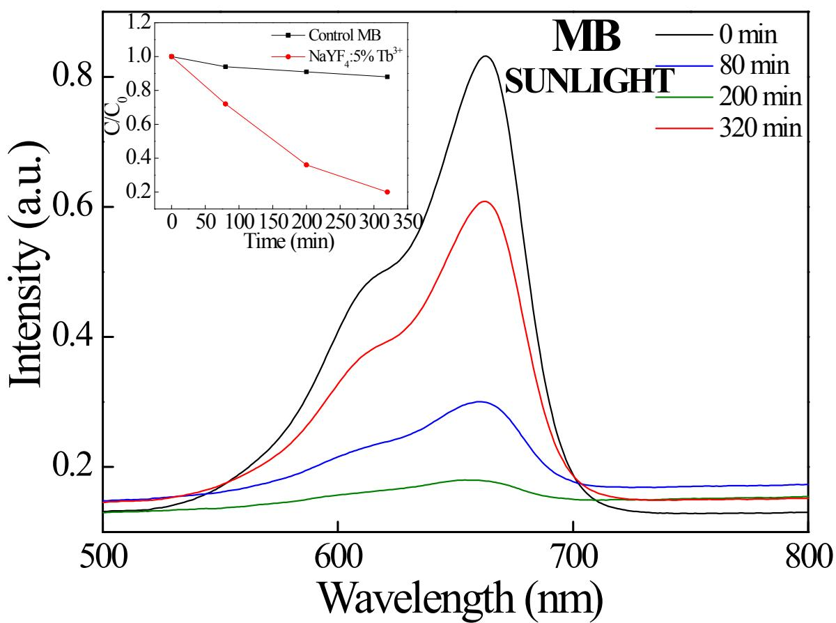
**Figure S3:** Photocatalytic degradation of MB in presence of  $\beta\text{-NaYF}_4:5\% \text{Tb}^{3+}$  under solar light irradiation. Inset showing corresponding plot of  $(C/C_o)$  vs. time.
