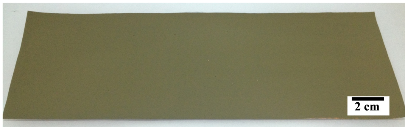
Figure S4. A digital photograph of a uniformly coated electrode film (7 cm × 23 cm) consisting of SiSMPs, Super P carbon black and 3D alginate network.
