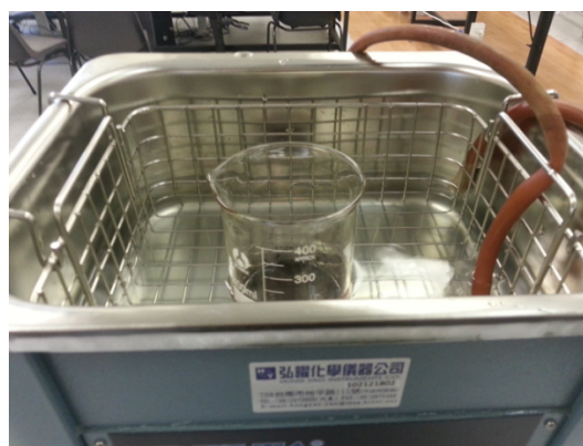
Fig. S1 Ultrasonication bath for simultaneously oxidizing and ultrasonication graphite (oxidi-sonication)
