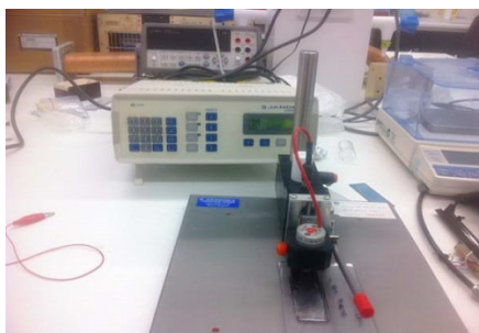
Fig. S7 Four-point probe used to test the surface resistivity (911 \Omega /square) of graphene films prepared by casting graphene suspension.
