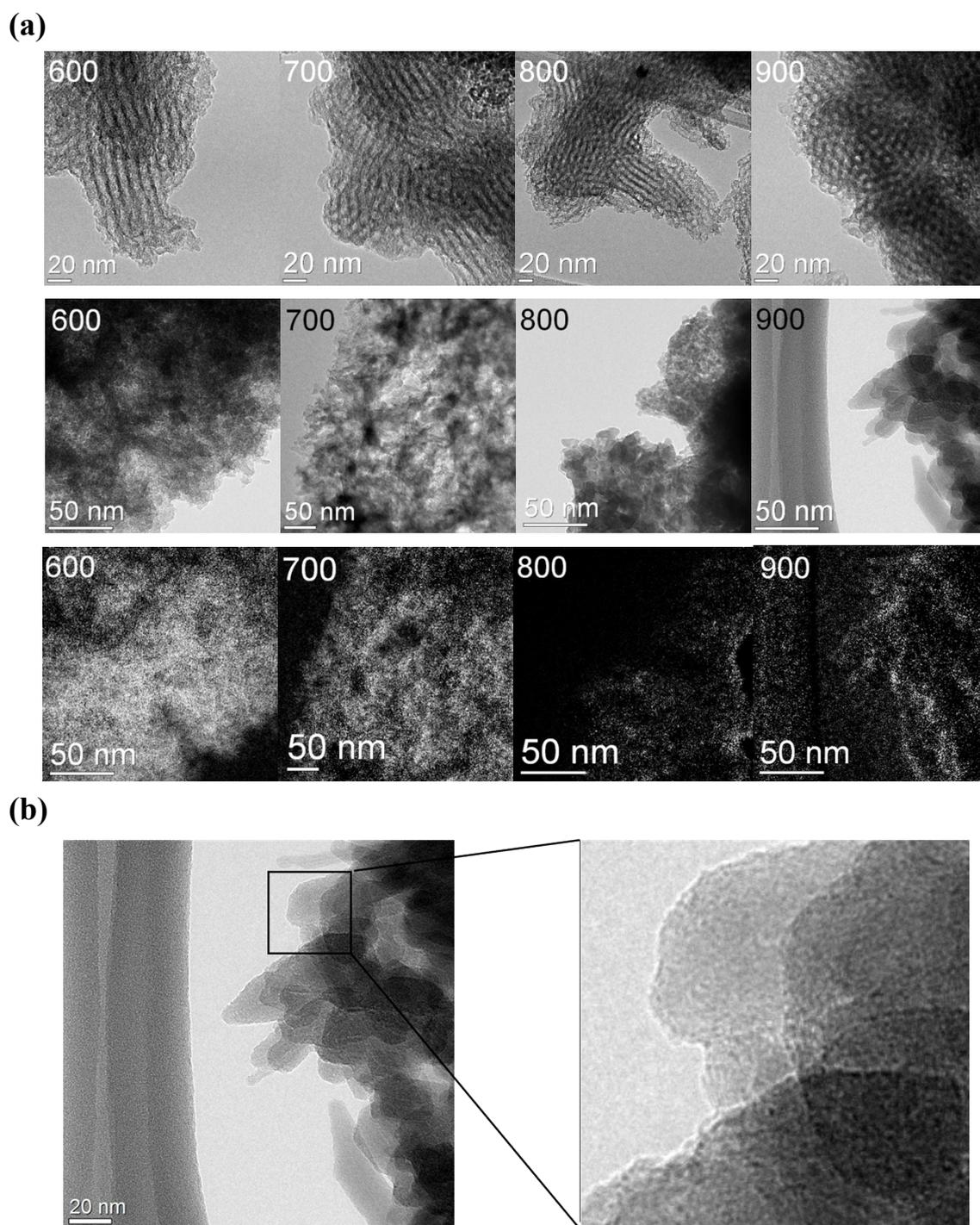
**Fig. S2** (a) TEM images of various C-Si-T (Top) and NMC-T (middle) materials with varied carbonization temperature  $T$  ranging from 600 to 900 °C. Bottom: EELS N-mapping images of NMC-Ts, and (b) enlarged TEM image of NMC-900
