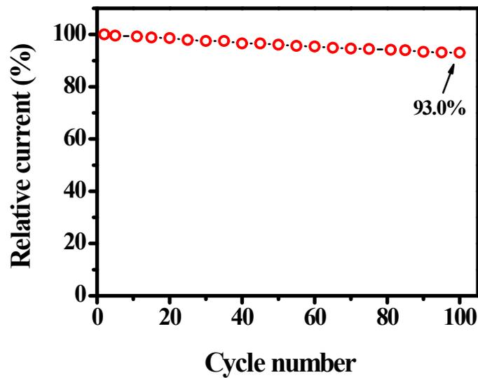
**Fig. S4** Durability of NMC-900 up to 100 CV cycles. Only assorted results are shown for clarity reason. Relative currents were calculated based on oxygen reduction peak at  $-0.26$  V.
