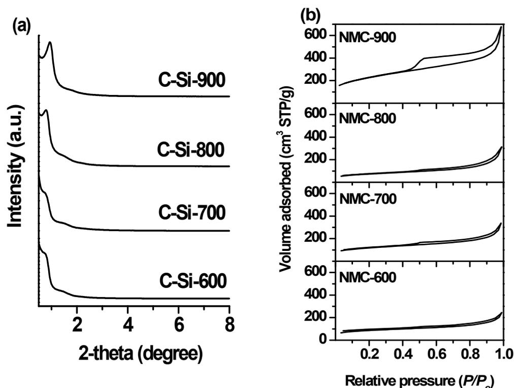
**Fig. S1** (a) Small-angle XRD patterns of N-doped C-Si-T composites and (b) N<sub>2</sub> adsorption/desorption isotherms of NMC-T samples prepared with different carbonization temperatures (T = 600, 700, 800, and 900 °C) under microwave irradiation.
