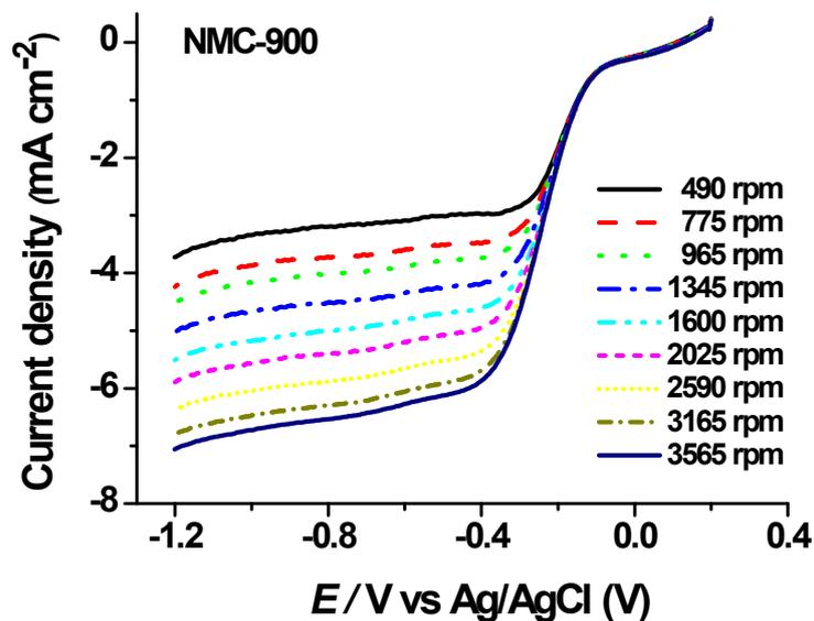
**Fig. S5** Rotating disk electrode (RDE) voltammograms of NMC-900 supported GCE in  $O_2$ -saturated  $0.1$  M KOH solution recorded at a scan rate of  $10$   $mV\ s^{-1}$  and varied rotation speeds ( $490 \sim 3565$  rpm).
