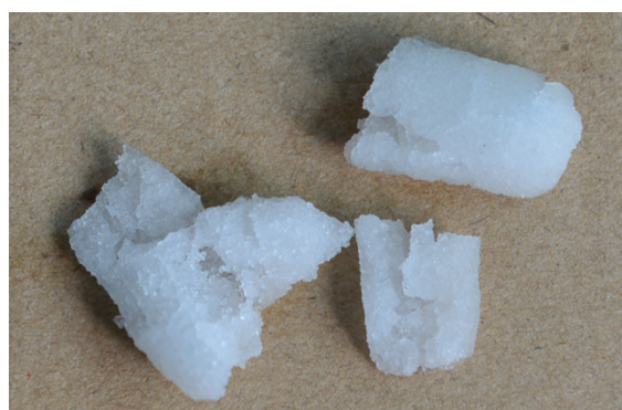
Fig. S1. Images of PDMS sponges (a) with embedded urea microparticles of different size after curing and washing ( m_{\text{PDMS}}/m_{\text{dimethicone}} = 4:6 ), (b) using n -hexane as the solvent ( m_{\text{PDMS}}/m_{\text{dimethicone}} = 6:4 , the size of NaCl microparticles is 150 ~ 297 \mu\text{m} ), and (c) using p -xylene as the solvent ( m_{\text{PDMS}}/m_{\text{dimethicone}} = 10:6:4 , the size of NaCl microparticles is 150 ~ 297 \mu\text{m} ).
