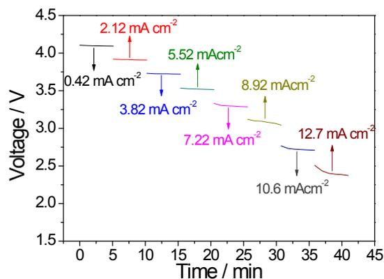
Figure S5. Discharge voltage curves in the current density range of 0.42 to 12.7 mA cm<sup>-2</sup>. At each current density, the test was carried out for 5 mins instead of several seconds.
