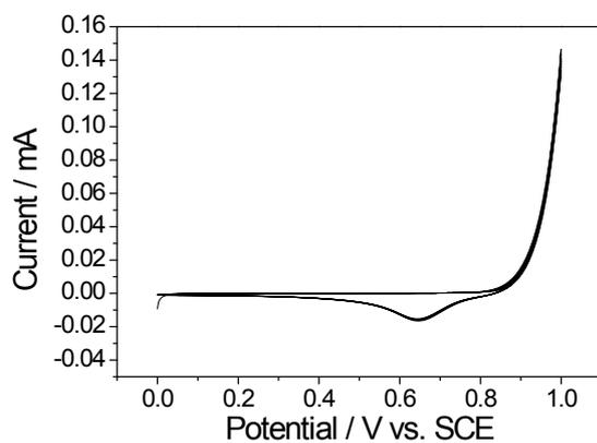
Figure S4. CV curves of 7 mol L<sup>-1</sup> LiBr aqueous solution at the scan rate of 0.5 mV s<sup>-1</sup> for the first 10 scans.
