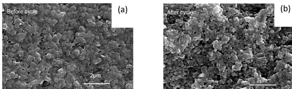
Figure S7. SEM micrographs of LISICON layer before and after 100 cycles at 35% depth of discharge.
