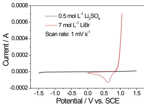
Figure S3. CV curves of the GC electrode in the aqueous solutions at the scan rate of 1 mV s<sup>-1</sup>.
