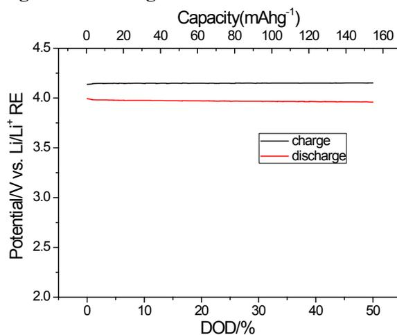
Figure S5. The charge /discharge curves for 100% DOD of the Li//Br battery in which aqueous positive electrode is 1 mol L<sup>-1</sup> LiBr with 0.1 mol L<sup>-1</sup> Br<sub>2</sub>.
