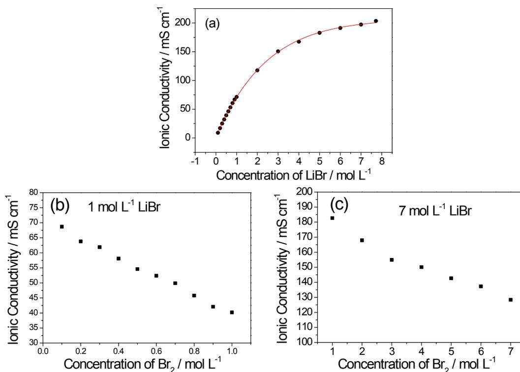
Figure S1. (a) Ionic conductivity of LiBr aqueous solution of different concentration, (b) and (c) ionic conductivities of 1 and 7 mol L<sup>-1</sup> LiBr aqueous solutions adding with different concentration of Br<sub>2</sub>.
