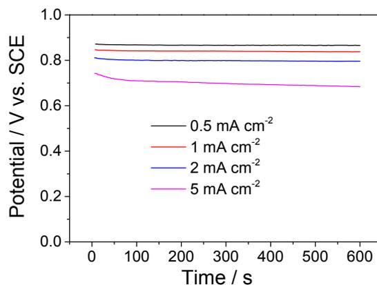
Figure S6. Discharge curves for Br single electrode (1 mol L<sup>-1</sup> Br<sub>2</sub>) in 7 mol L<sup>-1</sup> LiBr at different current densities.
