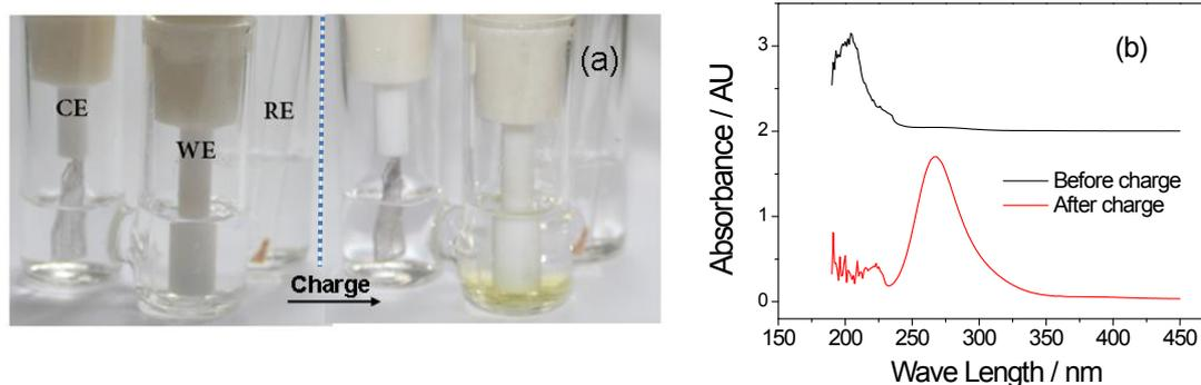
Figure S2. (a) Optical images of the solution around the GC electrode surface before and after a charge in 3 mol L<sup>-1</sup> LiBr aqueous solution, and (b) UV-Vis spectra of the solution before (black) and after (red) charge.
