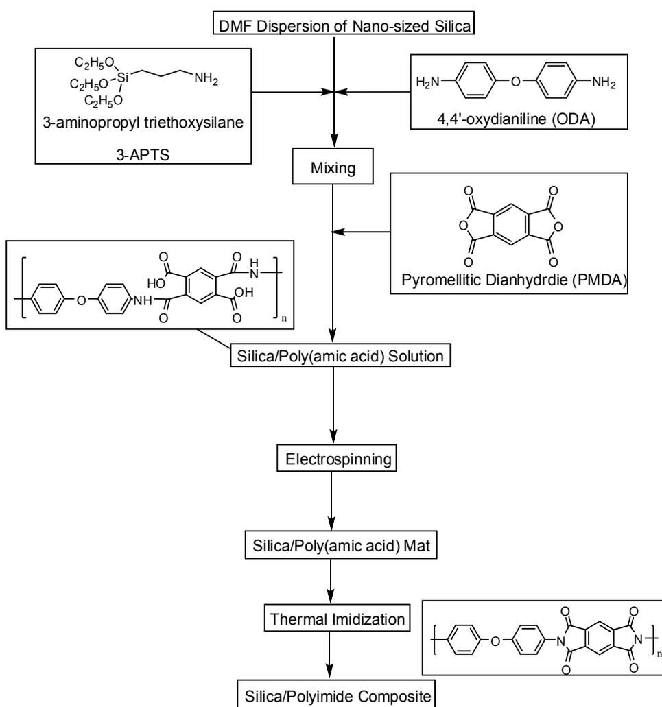
**Scheme S1. Synthetic route of PI and Silica/PI nanocomposite.**
