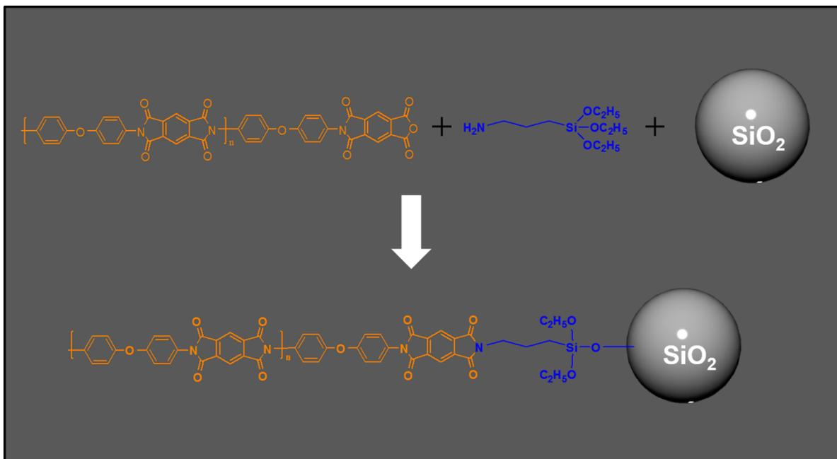
**Figure S4. The speculation of coupling mechanism of 3-APTS, based on Ref. [S1-S3].** The 3-APTS agent served as the coupling agent which linked between PI matrix and Silica particles. The amino group of 3-APTS attacked the anhydride ended polymer chain-tip while the other side bonded with the surface silica particles. Such chemical bondings enabled the silica particles to be firmly embeded on the polyimide surfaces.
