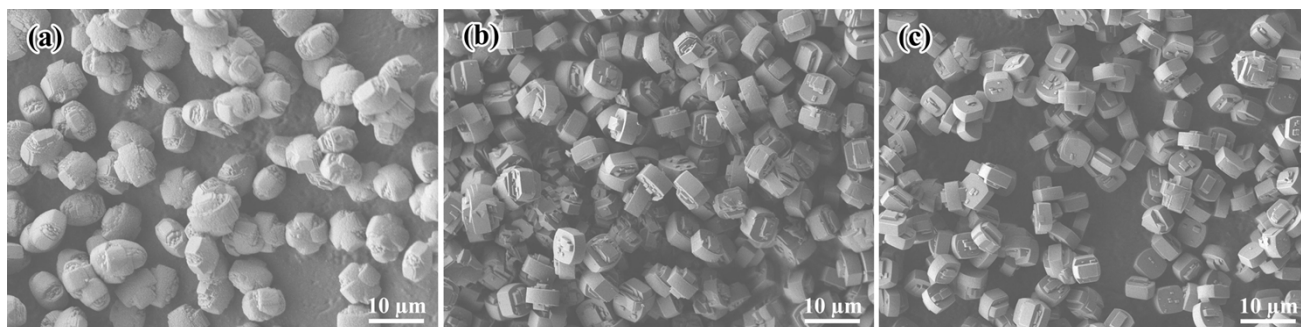
Figure S2 SEM image of the (a) CZS-30, (b) CZS-60 and (c) CZS-90, which demonstrate the conventional ZSM-5 is in micron level.
