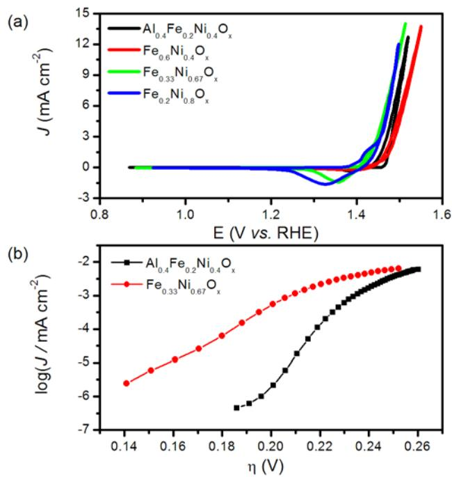
**Figure S5.** Cyclic voltammograms (after iR correction) of several Al/Fe/Ni series compositions deposited on FTO and recorded in 0.1 M KOH at a scanning rate of 10 mV s $^{-1}$ .
