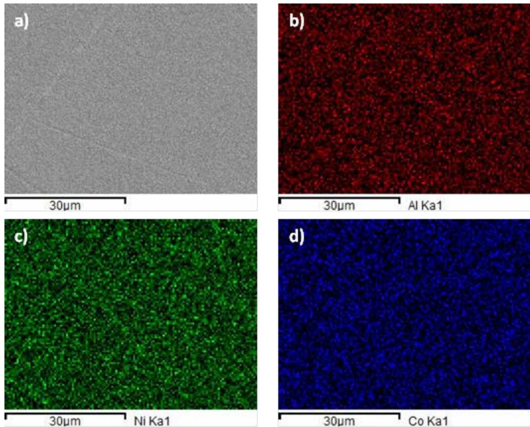
**Figure S4.** a) SEM image of an  $\text{Al}_{20}\text{Co}_{20}\text{Ni}_{60}\text{O}_x$  film on FTO and b)-d) EDXS elemental mapping images showing Al K  $\alpha_1$  (red), Ni K  $\alpha_1$  (green) and Co K  $\alpha_1$  (blue), respectively.
