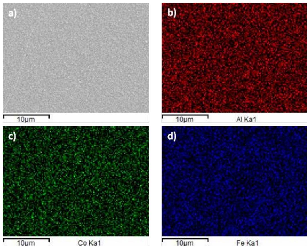
**Figure S3.** a) SEM image of an  $\text{Al}_{20}\text{Co}_{60}\text{Fe}_{20}\text{O}_x$  film on FTO and b)-d) EDXS elemental mapping images showing Al K  $\alpha_1$  (red), Co K  $\alpha_1$  (green) and Fe K  $\alpha_1$  (blue), respectively.
