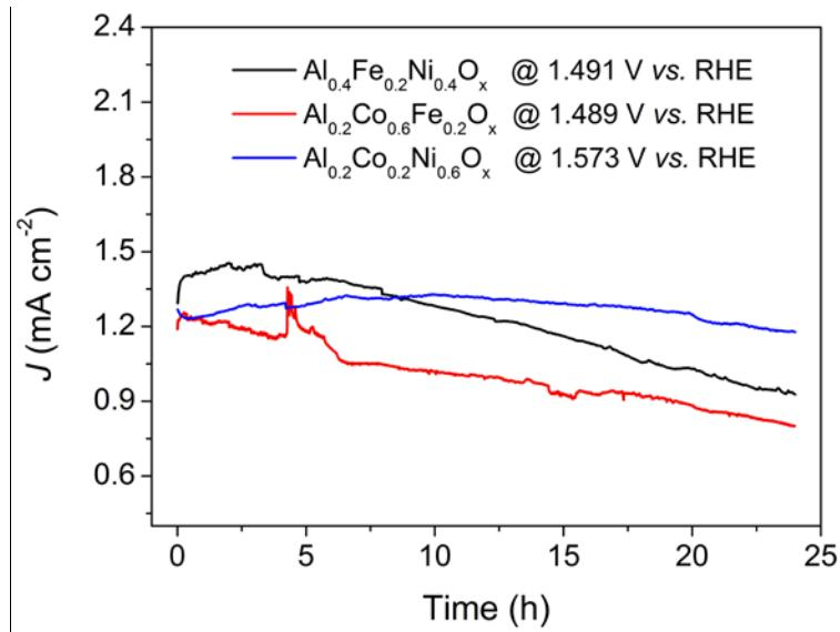
**Figure S8.** Temporal stability of  $\text{Al}_{0.4}\text{Fe}_{0.2}\text{Ni}_{0.4}\text{O}_x$ ,  $\text{Al}_{0.2}\text{Co}_{0.6}\text{Fe}_{0.2}\text{O}_x$ ,  $\text{Al}_{0.2}\text{Co}_{0.2}\text{Ni}_{0.6}\text{O}_x$  in 0.1 M KOH at 25 °C.
