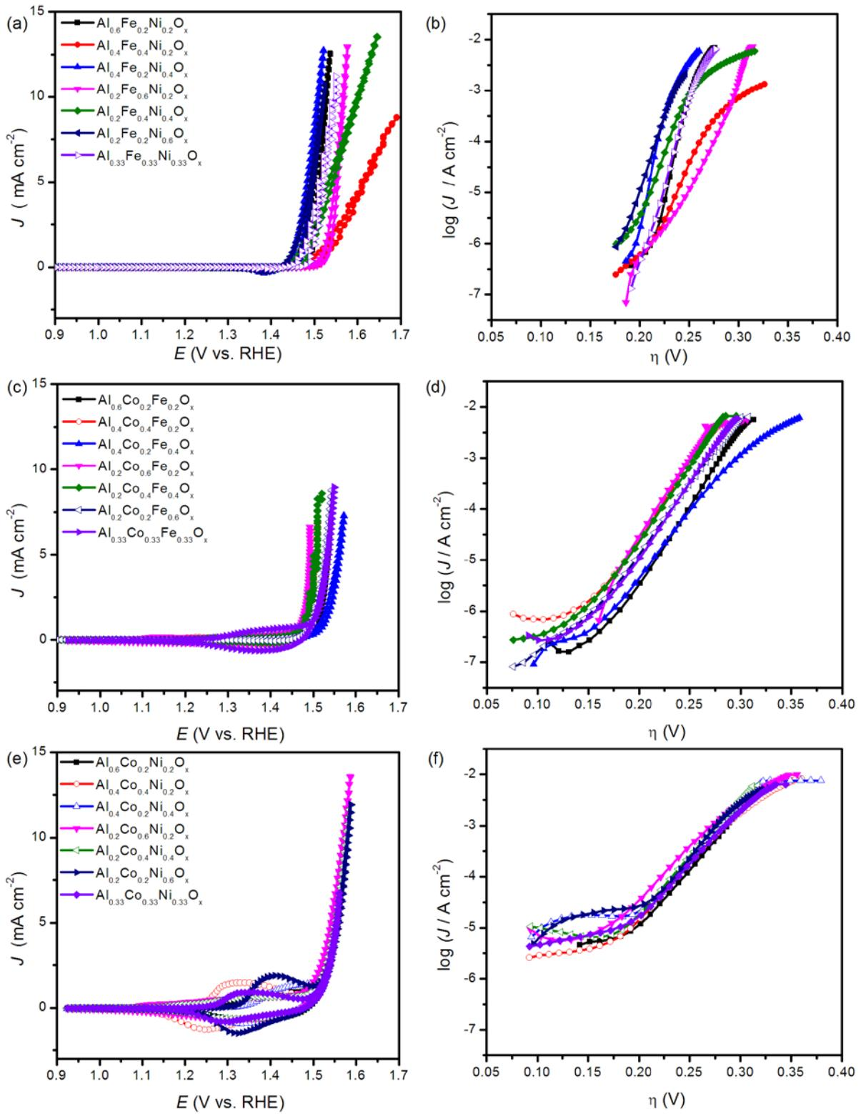
**Figure S6.** Cyclic voltammograms (left column) and Tafel plots (right column) of (a-b) Al/Fe/Ni, (c-d) Al/Co/Fe, and (e-f) Al/Co/Ni ternary metal oxide films in 0.1 M KOH.
