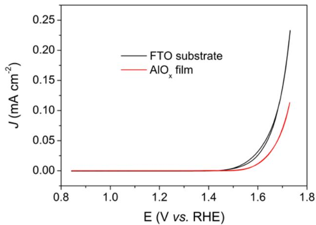
**Figure S7.** Cyclic voltammograms for aluminum oxide deposited on FTO, and the bare FTO substrate itself (recorded in 0.1 M KOH at a scanning rate of 10 mV s<sup>-1</sup>).
