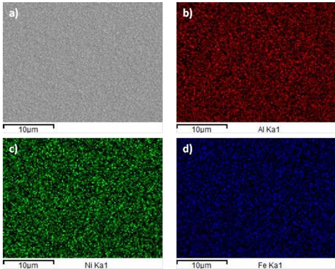
**Figure S2.** a) SEM image of an  $\text{Al}_{40}\text{Fe}_{20}\text{Ni}_{40}\text{O}_x$  film on FTO and b)-d) EDXS elemental mapping images showing Al K  $\alpha_1$  (red), Ni K  $\alpha_1$  (green) and Fe K  $\alpha_1$  (blue), respectively.
