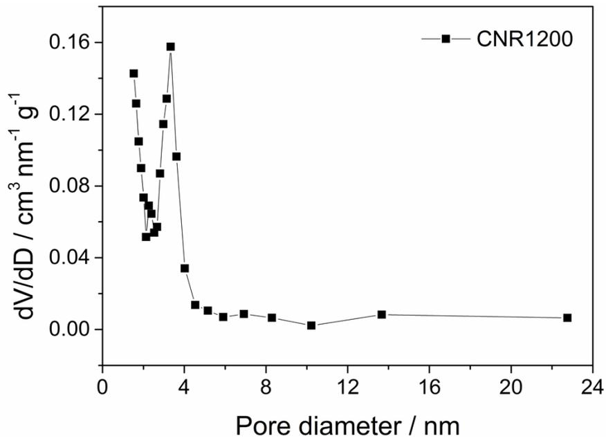
**Fig. S2.** Pore size distribution of CNR1200.
