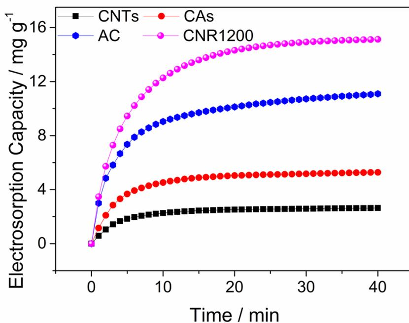
**Fig. S3.** Electrodesorption capacities for AC, CNTs, CAs and CNR1200 electrodes in NaCl solutions with an initial concentration of 500 mg l<sup>-1</sup>.
