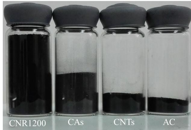
**Fig. S1.** The comparison of densities between CNR1200, CAs, CNTs and AC powders (1 g power in each vial).
