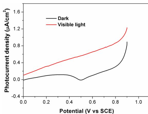
**Fig. S2** Linear-sweep voltammograms of the  $\text{Fe}_2\text{O}_3$  film electrode collected with a scan rate of  $10 \text{ mV} \cdot \text{s}^{-1}$  in dark and under visible light illumination in  $0.5 \text{ M Na}_2\text{SO}_4$  aqueous solutions.
