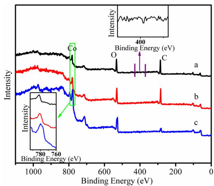
**Figure S2** XPS spectrums of the  $\text{Co}_3\text{O}_4$ @MWCNT (black line a),  $\text{Co}_3\text{O}_4$ -MWCNT (red line b) and  $\text{Co}_3\text{O}_4$  (blue line c). The inset of line a for  $\text{Co}_3\text{O}_4$ @MWCNT around 400 eV shows high resolution of the N region between two purple lines, and no significant signals are found in the N1s region, while another inset is the enlarged figure around 780 eV.
