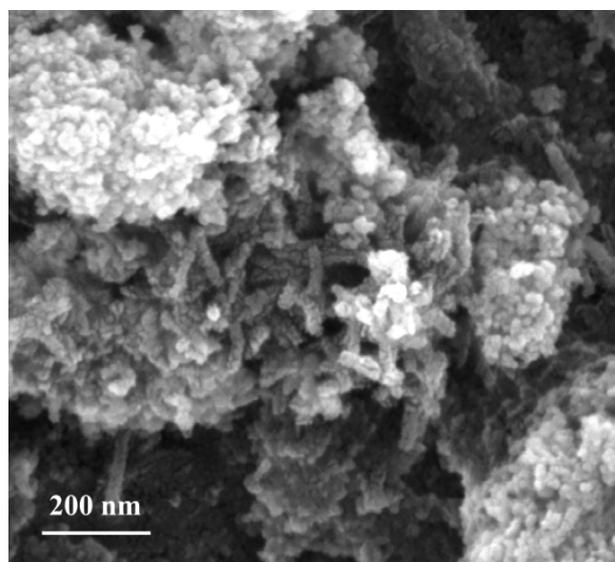
**Figure S1** SEM image of the  $\text{Co}_3\text{O}_4$ -MWCNT hybrid synthesized with raw MWCNT.
