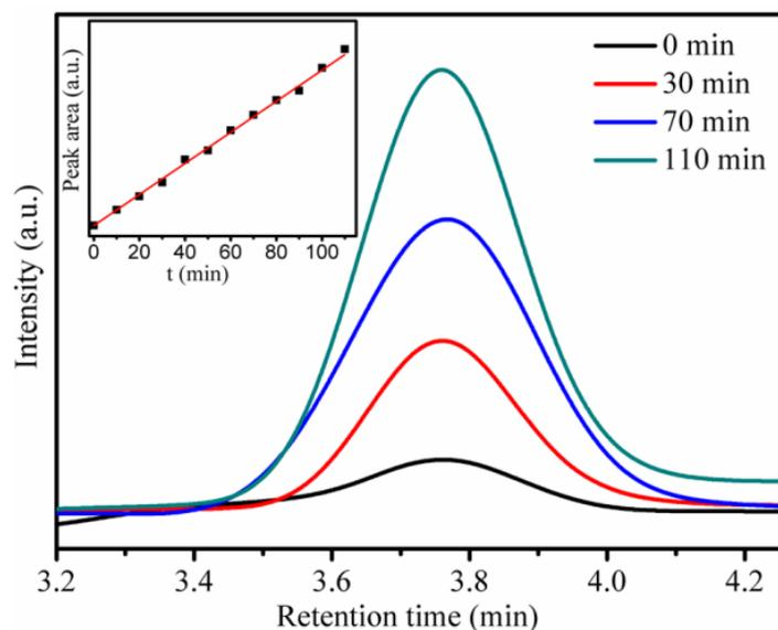
**Figure S5** Gas chromatograph of oxygen obtained by ITO modified with  $\text{Co}_3\text{O}_4@\text{MWCNT}$  under electrolysis at 0.8 V vs. Ag/AgCl, the inset is the oxygen integral areas as a function of time.
