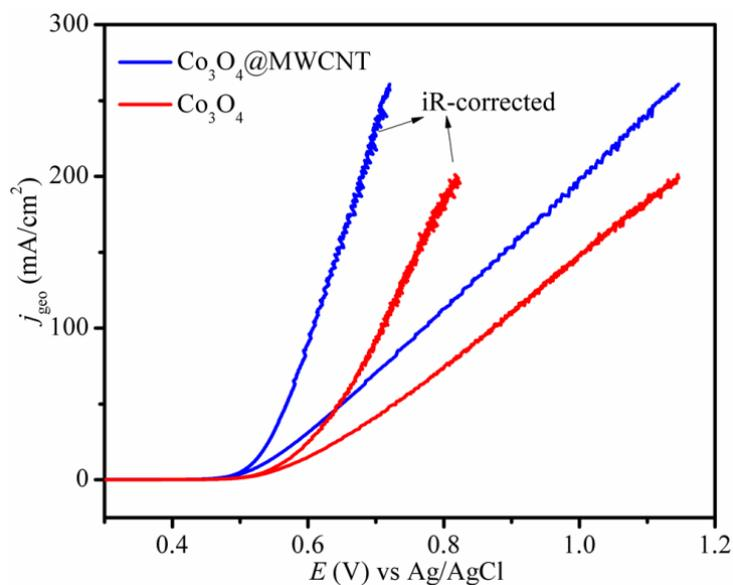
**Figure S3** LSVs for modified GC electrodes comprising the  $\text{Co}_3\text{O}_4$  nanorods and nanocubes, respectively, with and without iR correction. 1M KOH,  $R_{\text{Co}_3\text{O}_4@\text{MWCNT}} = 6.2 \Omega$ ,  $R_{\text{Co}_3\text{O}_4} = 6.6 \Omega$ .
