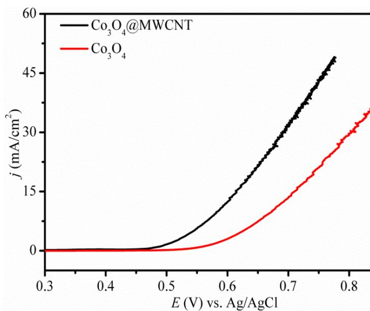
**Figure S4** Linear sweep voltammetry curves (LSVs) obtained with RDE modified with  $\text{Co}_3\text{O}_4@\text{MWCNT}$  hybrid and  $\text{Co}_3\text{O}_4$  respectively (after IR compensation) in 0.1 M KOH, Experimental conditions: the  $j$  ( $\text{mA cm}^{-2}$ ) is normalized by geometric area of the glassy carbon electrode, T: 298 K, glassy carbon electrodes of RDE at 2000 rpm, Scan rate:  $1 \text{ mV s}^{-1}$ .
